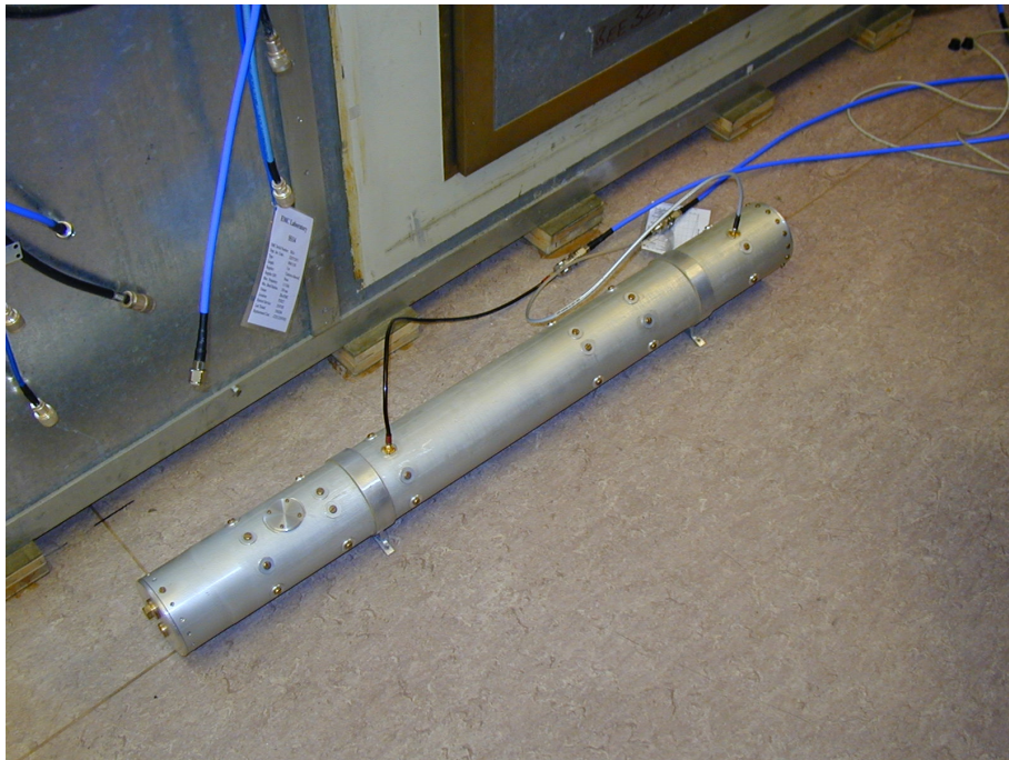
Figure 4.5: The metal cylinder used to demonstrate waveguide effects
