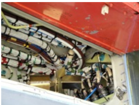
Figure 7.4: Stirrer and one antenna for the first single bay measurement
