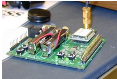
Figure 4.4: A Jennic ZigBee unit as used for the first measurements
