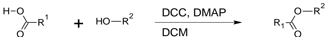
Figure 3-1 General scheme of the Steglich esterification reaction between carboxylic acid and alcohol using the DCC/DMAP coupling system.
