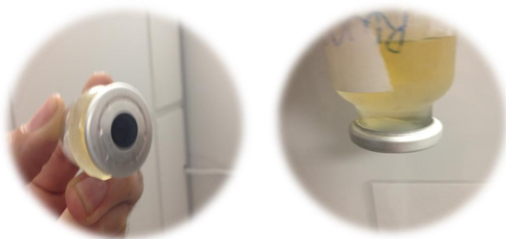
Figure 3.10: Pictures for the airtight vials used to storage the withdrawal samples.
