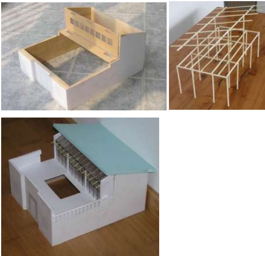
Fig. 8.16 Models from the barefoot-architect became a key medium to communicate and collaborate with local carpenters and masons. Top left: wall-enclosure model; Top right: wood structure model; bottom: 'final' model with roof articulations. (Photograph by Weizhong Ren)
