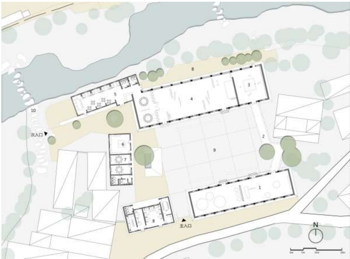
Fig. 4.7 Ground Floor Plan (Drawn by Wei He)
