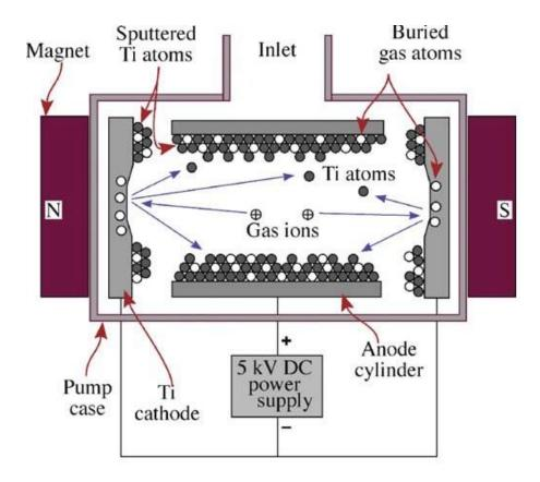
Figure 3.3: Schematic diagram of an ion pump [1].
