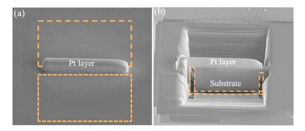
Figure 3.15: (a) Shows the deposited Pt on the sample surface. The orange dashed lines show the regions that the trenches are going to be sputtered out. (b) Shows the region of interest after the trenches have been milled out. The orange dashed lines show the regions of the U cut before the lift-out.
