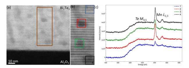
Figure 5.5: (a) Low magnification HAADF-STEM image of the  $Bi_2Te_3$  film and the  $Al_2O_3$  substrate. (b) HAADF-STEM signal from the region of interest outlined in (a). (c) Background-subtracted Mn  $L_{2,3}$  and Te  $M_{4,5}$  edges extracted from the regions shown in (b). Spectra have been shifted vertically for clarity.
