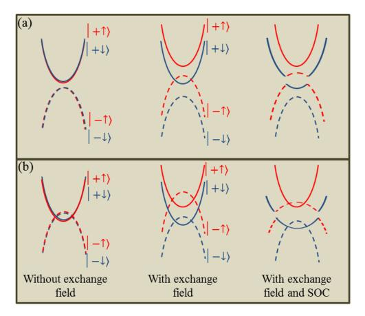
Figure 2.12 Evolution of the subband structure upon the increase of the exchange field. The solid and dashed lines show the subbands that have even and odd parity at  $\Gamma$  point, respectively.
