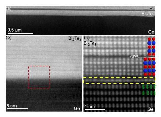
Figure 7.2: (a) Overview HAADF-STEM image of the  $Bi_2Te_3$  film on Ge(111). (b) Magnified HAADF-STEM image from the interface region. (c) High-magnification HAADF-STEM image from the interfacial region between the  $Bi_2Te_3$  film and the Ge outlined in (b). The overlaid structural model and the dashed rectangle show the  $Bi_2Te_3$ /Ge atomic positions as well as the extra layer at the interface; Bi (blue), Te (red), and Ge (green) atomic columns.
