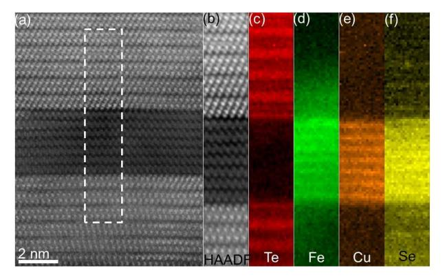
Figure 6.3: (a) HAADF-STEM survey image from the  $Bi_2Te_3$  film and the  $Fe_xCu_{1-x}Se$  inclusion. (b) HAADF-STEM signal from the region outlined by a dashed rectangle in (a), obtained simultaneously with the EELS data. (c-f) show Te  $M_{4,5}$ , Fe  $L_{2,3}$ , Cu  $L_{2,3}$ , and Se  $L_{2,3}$  EELS signals at the  $Fe_xCu_{1-x}Se/Bi_2Te_3$  interface, respectively.
