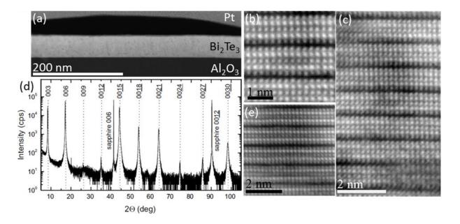
Figure 5.1: (a) Low magnification HAADF-STEM image of the  $Bi_2Te_3$  film on  $Al_2O_3$  (0001) substrate. (b), (c), and (e) are atomically resolved HAADF-STEM images of different places of the  $Bi_2Te_3$  film. Good crystalline QL structure of the  $Bi_2Te_3$  film is present. (d) XRD diagram showing both film and substrate peaks as labelled.
