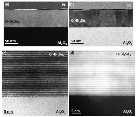
Figure A1: (a) and (b) show HAADF and BF-STEM images of the Cr doped Bi<sub>2</sub>Se<sub>3</sub>. (c) and (d) show high magnification HAADF and BF-STEM images of the Cr doped Bi<sub>2</sub>Se<sub>3</sub> sample. QL structure of Bi<sub>2</sub>Se<sub>3</sub> can be seen in (c) and (d).
