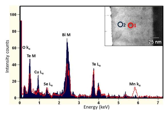
Figure A4: Shows the energy-dispersive X-ray spectrums of two positions inside the Mn doped  $Bi_2Te_3$  sample. The red line and filled blue spectrums correspond to points 1 and 2 in the HAADF-STEM image shown as an inset, respectively. From the peak intensities, it is clear that the dark patch (point 1) is higher in Mn and lower in Te and Bi, comparing to the second sampling area (point 2).
