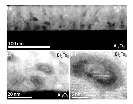
Figure 5.8: (a) Low magnification HAADF-STEM image of the  $Bi_2Te_3$  film and the  $Al_2O_3$  substrate with  $\sim$  6 at-% of Mn doping. (b) Shows the regions of the film with dark patches. (c) Shows higher magnification image of the patch area forming secondary phases with deteriorated crystallinity.
