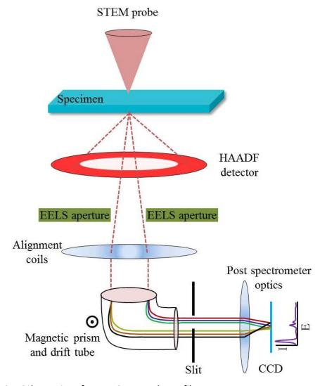
Figure 3.27: Schematics of an EELS post column filter.
