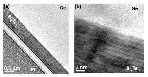
Figure A6: (a) and (b) show the overview and high magnification TEM images of the Bi<sub>2</sub>Te<sub>3</sub> on the Ge substrate.
