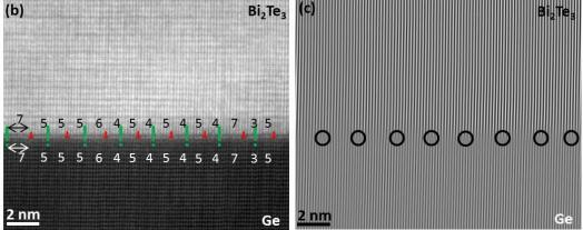
Figure A7: (a) and (b) show the HAADF-STEM images of the Bi<sub>2</sub>Te<sub>3</sub> film on the Ge substrate with the ML of Te at the interface. (c) HAADF-STEM image masked to only show the vertical planes reveals the misfit dislocations at the interface. The green and red features on (b) show the position of not stressed and stressed atomic planes with their corresponding number of atomic planes in-between them, respectively.
