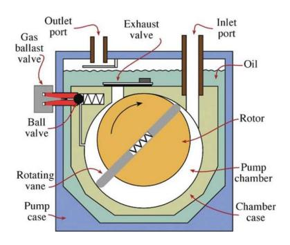
Figure 3.1: Cross-section of a rotary pump [1].
