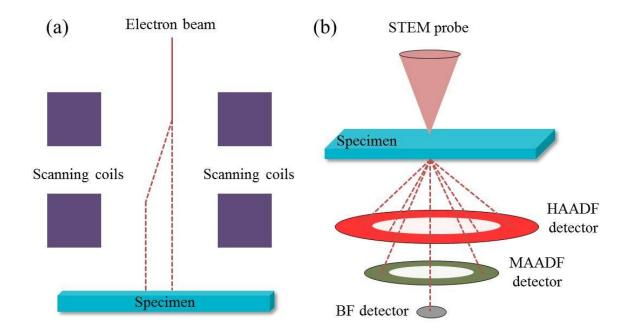
Figure 3.24: (a) shows schematic of the scanning coils above the specimen in STEM and (b) shows the HAADF, MAADF, and the BF detectors presence below the specimen.
