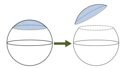
Figure 2.5: The loop divides the surface into two areas with the same boundary. The magnetic flux through both areas changes by multiple of  $^h/_e$  so the total flux of the sphere is quantised in the units of flux quanta.
