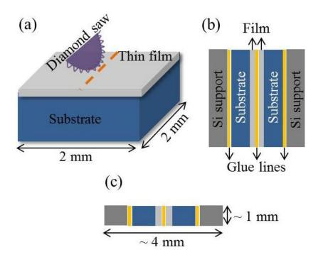
Figure 3.9: (a) Schematic of the specimen in the cutting step. (b) Top view schematic of the specimen ready to be mechanically polished. (c) Side view schematic of the specimen showing the 1 mm thickness of the sample before the mechanical polishing.
