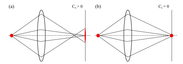
Figure 3.20: (a) and (b) show the schematics of imaging a point object using an electromagnetic lens with and without having spherical aberration, respectively.
