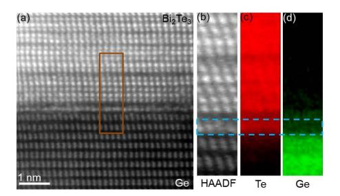
Figure 7.3: (a) HAADF-STEM survey image. (b) HAADF-STEM signal from the region of interest outlined in (a) produced simultaneously with the EELS acquisition. (c) and (d) Te  $M_{4,5}$  and Ge  $L_{2,3}$  EELS signals showing the presence of Te in the observed extra layer (outlined by a dashed blue rectangle).
