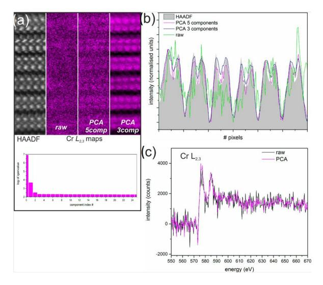
Figure 4.9: (a) HAADF-STEM signal, Cr  $L_{2,3}$  intensity maps (raw and treated by PCA, respectively) and Scree plot, (b) integrated intensity profiles of the HAADF signal and Cr  $L_{2,3}$  maps corresponding to (a). (c) Background subtracted Cr  $L_{2,3}$  EELS edge before and after PCA (3components) showing the reduction of noise.
