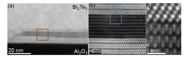
Figure 6.2: (a) Overview image of the  $Fe_xCu_{1-x}Se$  inclusion close to the  $Bi_2Te_3/Al_2O_3$  interface. (b) Magnified HAADF-STEM image from the region of interest outlined in (a). Both the film and the  $Fe_xCu_{1-x}Se$  inclusion show good crystallinity. (c) High-magnification HAADF-STEM image from the interfacial region between the  $Bi_2Te_3$  film and the  $Fe_xCu_{1-x}Se$  outlined in (b).
