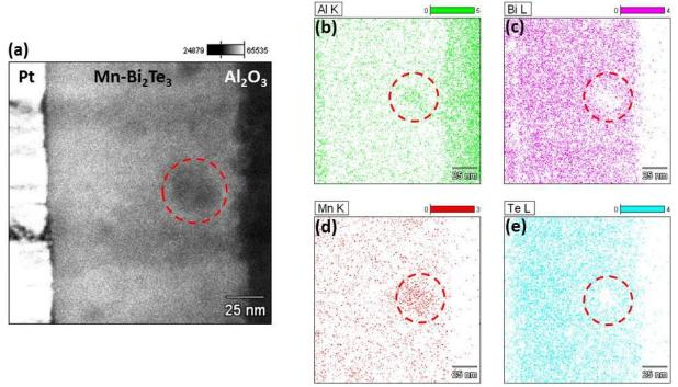
Figure A3: (a) Shows HAADF-STEM image of a dark patch inside the Mn doped  $Bi_2Te_3$  sample. (b), (c), (d), and (e) show the energy-dispersive X-ray spectroscopy maps of Al, Bi, Mn, and Te, respectively.
