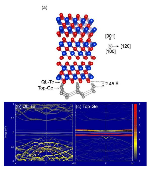
Figure 7.6: (a) Structure of  $3QL-Bi_2Te_3/Ge(111)$  and band structures for (b) QL-Te and (c) top-Ge. The notations are the same as in **Figure 7.5**.
