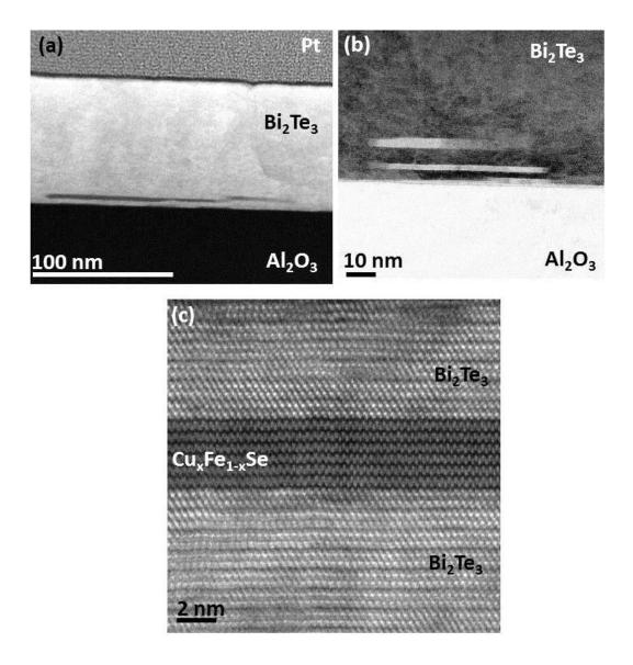
Figure A5: (a) and (b) show the HAADF and BF-STEM images of  $Fe_xCu_{1-x}Se$  within the  $Bi_2Te_3$  TI. The dark and bright areas inside the  $Bi_2Te_3$  film in (a) and (b) show the  $Fe_xCu_{1-x}Se$  inclusions, respectively.
