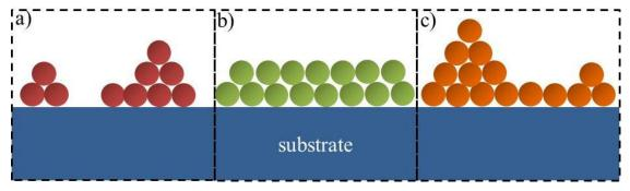
Figure 3.5: Three different growth mods of island, layer by layer, and mixed growth are shown in (a), (b), and (c), respectively.
