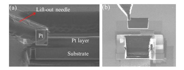
Figure 3.16: (a) Shows the deposited Pt to fix the lamella to the lift-out needle. (b) Shows the lamella after the full cut out.
