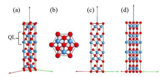
Figure 2.11: (a) Crystal structure of  $Bi(Sb)_2Se(Te)_3$ . (b), (c), and (d) show the crystal structure in (0001), the (11 $\overline{2}$ 0), and (10 $\overline{1}$ 0), respectively.
