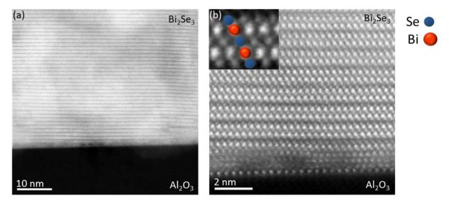
Figure 4.5: (a) HAADF-STEM overview image from the interfacial region between the film and substrate. (b) Magnified image of the film at the interface. A smooth interface and regular Bi<sub>2</sub>Se<sub>3</sub> QLs are found, except for the first layer which appears to be highly disordered. The inset shows magnified image of a QL with overlaid structural model; Bi (red) and Se (green) atomic columns.
