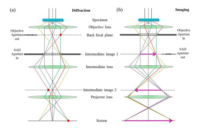
Figure 3.22: (a) and (b) show schematics of the lenses and apertures in diffraction and imaging mode, respectively.
