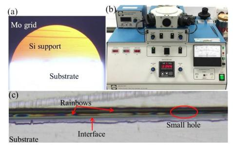
Figure 3.10: (a) Yellow colour of the Si support under the optical microscope in transmission mode. (b) The ion milling machine. (c) The rainbows and the hole at the interface glue line from Ar ion milling.
