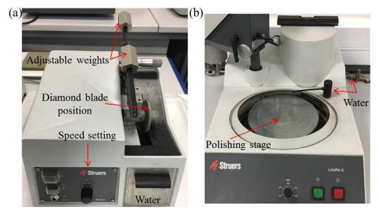
Figure 3.8: (a) Wafer cutting machine and its relevant components. The weights are used to counterbalance the weight of the sample which tunes the cutting speed. The water is used to clean the diamond blade continuously while cutting. (b) The polishing stage. The water is used to continuously clean the polishing pads while the specimen is being polished.
