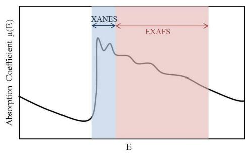
Figure 3.7: XAS absorption coefficient vs. energy plot showing XANES and EXAFS.
