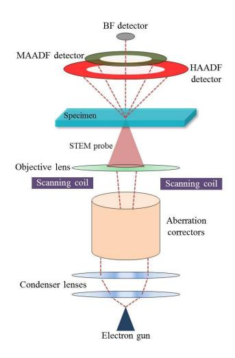
Figure 3.25: Simplified schematic of a STEM microscope.
