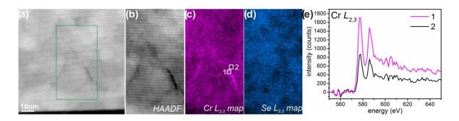
Figure 4.7: (a) HAADF-STEM survey image. (b) HAADF-STEM signal from the region of interest outlined in (a) produced simultaneously with the EELS acquisition. (c) Cr  $L_{2,3}$  EELS signal showing Cr segregation along the grain boundaries. (d) Se  $L_{2,3}$  EELS signal showing uniform distribution of Se in the film. (e) Cr  $L_{2,3}$  edges obtained from the grain boundary and off boundary regions labeled as number 1 and 2 in (c), showing enhanced Cr signal at the grain boundary.
