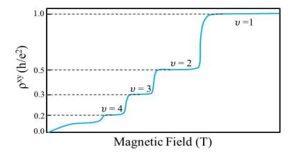
Figure 2.2: Illustration of the Hall resistivity plotted as a function of applied field.  $\rho^{xy}$  plateaus at  $h/ve^2$  in a quantum Hall phase.
