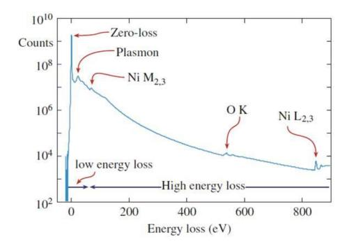
Figure 3.28: EELS map of NiO specimen showing the zero loss, low loss, and the core loss regions as well as the plasmon peak [1].
