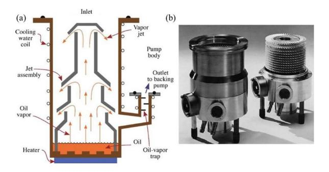
Figure 3.2: (a) Cross-section of a diffusion pump [1]. (b) Turbomolecular.
