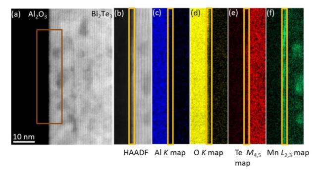
Figure 5.6: (a) HAADF-STEM survey image in which the region selected for simultaneous acquisition of EELS for elemental mapping is highlighted. (b) Magnified HAADF image outlined with brown rectangle in (a). The elemental Al, O, Te, and Mn maps are shown in (c), (d), (e), and (f), respectively. Al and Te elemental maps in (c) and (e) show no intermixing between substrate and film. The Mn elemental map (f) shows the segregation of Mn at the interface.
