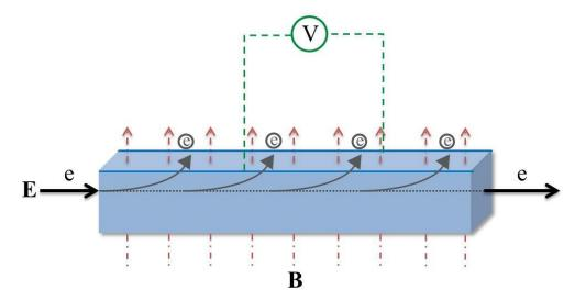
Figure 2.1: Hall setup showing measured voltage that arises from deflected motion of charged particles in solids under external electric (E) and magnetic fields (B).
