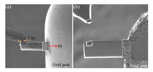
Figure 3.17: (a) Show the deposited Pt which fixed the lamella to the grid as well as the cutting point for removing the needle. (b) Shows the lamella fixed to the grid and the cut outed lift-out needle.
