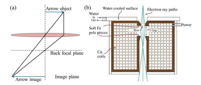
Figure 3.19: (a) Schematic of a conventional optical lens. (b) Cross-sectional schematic diagram of a magnetic lens [1].
