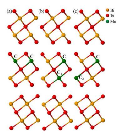
Figure 5.10: Simulation models for  $Bi_2Te_3$  with Mn atoms substituting Bi. (a) Shows two Mn atoms occupying the two nearest Bi atoms denoted as C. (b) Shows the Mn atoms occupying the closest Bi sites in two different planes of the  $Bi_2Te_3$  QL (C and  $C_1$ ). (c) Shows the Mn atoms occupying the furthest Bi sites in two different planes of the  $Bi_2Te_3$  QL (C and  $C_2$ ). The Bi, Te, and Mn atoms are represented by yellow, red, and green spheres, respectively.
