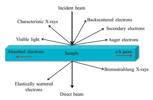
Figure 3.21: Schematic diagram of the main signals generated as an electron beam interacts with sample.
