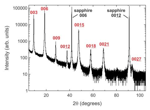
Figure 4.4: XRD of the Cr doped thin film using for this investigation. The film peaks are labeled in red and the sapphire substrate peaks in black.
