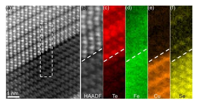
Figure 6.4: (a) HAADF-STEM survey image from the interface between the  $Bi_2Te_3$  film and the  $Fe_xCu_{1-x}Se$  inclusion. (b) HAADF-STEM signal from the interface region outlined by the dashed rectangle in (a), obtained simultaneously with the EELS data. (c-f) show Te  $M_{4,5}$ , Fe  $L_{2,3}$ , Cu  $L_{2,3}$ , and Se  $L_{2,3}$  EELS signals at the  $Fe_xCu_{1-x}Se/Bi_2Te_3$  interface, respectively.
