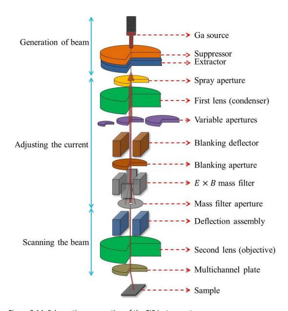
Figure 3.14: Schematic cross-section of the FIB instrument.
