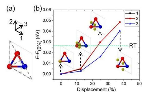
Figure 6.7: (a) Top view image of the  $Bi_2Te_3$  unit-cell. The grey dashed lines show the positions of which 32 different sampling has been done for the Se bonding energy calculations. (b) Relative energy variations along the three main crystallographic paths outlined in (a). The green dashed line shows the corresponding energy at room temperature (0.0257 eV).
