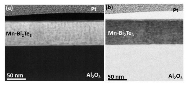
Figure A2: (a) and (b) show low magnification HAADF and BF-STEM images of the Mn doped Bi<sub>2</sub>Te<sub>3</sub>.
