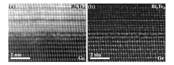
Figure 3.26: (a) and (b) show HAADF and BF-STEM images of the Bi<sub>2</sub>Te<sub>3</sub> on Ge substrate.
