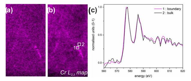
Figure 4.8: EELS maps of the Cr  $L_{2,3}$  edge produced using (a) raw and b) PCA treated data respectively., showing enhanced Cr signal at the grain boundary. The map in (b) corresponds to the map showing in Figure 7c. (c) background-subtracted Cr  $L_{2,3}$  edge extracted from the grain boundary and bulk regions (same as **Figure 4.7e**), normalized to the maximum of the  $L_3$  peak.
