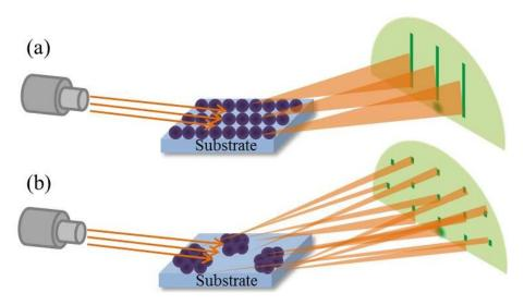
Figure 3.6: Schematics of RHEED pattern from (a) a flat surface and (b) a 3D nucleated surface. We note that the patterns appear on the screens are the superposition of the diffracted electrons wavefunctions.
