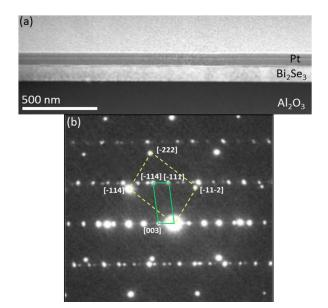
Figure 4.1: (a) Low magnification HAADF-STEM image of the  $Bi_2Se_3$  film on  $Al_2O_3$  (0001). (b) SAED from the  $Bi_2Se_3/Al_2O_3$  interface region along the  $[11\bar{2}0]$  crystallographic direction. The dashed (yellow) and solid (green) rectangles are showing the projected unit cells of  $Al_2O_3$  and  $Bi_2Se_3$ , respectively.
