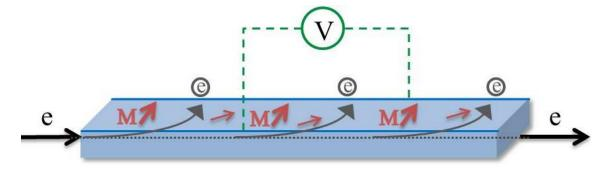
Figure 2.7: Illustration of anomalous Hall effect. The red arrows showing the magnetization (M) inside the sample.
