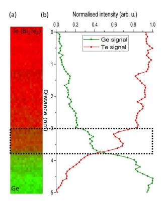
Figure 7.4: (a) and (b) show the overlaid maps of Te and Ge as well as their signal intensity profile across the area outlined in **Figure 7.3a**. Red and Green correspond to Te and Ge, respectively.
