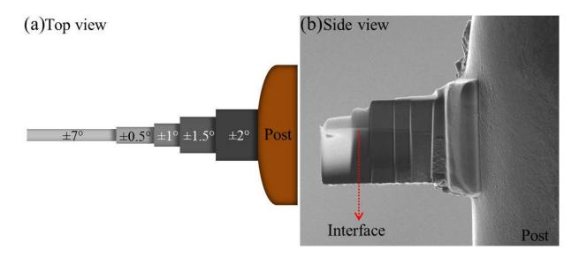
Figure 3.18: (a) Shows the schematic top view of the thinning steps. (b) Shows a side view SEM image of the thinning steps.
