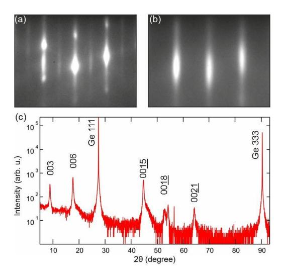
Figure 7.1: (a) and (b) show RHEED patterns obtained from the Ge and the  $Bi_2Te_3$  surfaces, respectively. (c) XRD spectrum showing both film and substrate peaks as labelled.
