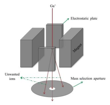
Figure 3.13: Schematic of the  $\boldsymbol{E} \times \boldsymbol{B}$  mass filter used in FIB instruments.
