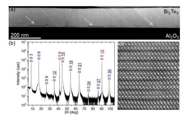
Figure 6.1: (a) Low-magnification HAADF-STEM image of the  $Bi_2Te_3$  film on the  $Al_2O_3$  substrate. The dashed arrows outline the  $Fe_xCu_{1-x}Se$  inclusions in the  $Bi_2Te_3$  film. (b) XRD spectrum showing both  $Al_2O_3$  substrate (red labels) and  $Bi_2Te_3$  film peaks (blue labels). (c) Atomically resolved HAADF-STEM image shows the QL structure of the  $Bi_2Te_3$  film.
