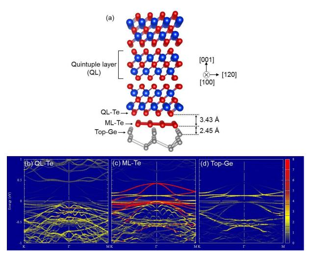
Figure 7.5: (a) The structure of  $3QL-Bi_2Te_3/Te/Ge(111)$ . Blue, red, and gray circles indicate Bi, Te, and Ge atoms, respectively. (b)-(d) Calculated band structures with weights of p orbitals along the  $K \to \Gamma \to M$  direction in the BZ for Te at the bottom of the  $QL-Bi_2Te_3$  (QL-Te), Te in the inserted monolayer (ML-Te), and Ge at top of Ge substrate (top-Ge), respectively.
