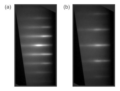
Figure 4.3: RHEED images of the Cr doped  $Bi_2Se_3$  film recorded in-situ at the end of the film growth along the (a)  $[10\overline{1}0]$  and (b)  $[11\overline{2}0]$  azimuths, respectively.
