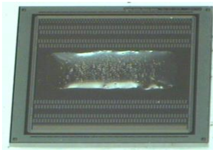
Figure 3-7 HPK Mini Silicon Sensor used in glue trials [65]
