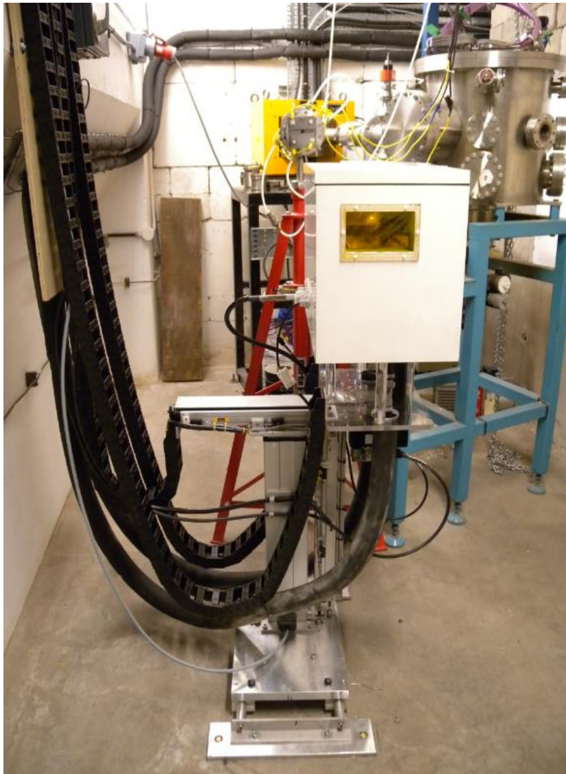
Figure 3-36 Upgraded cold box and robotic scanning systems [99]
