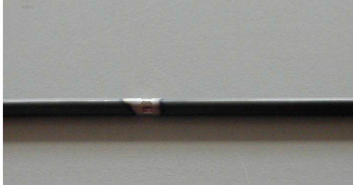
Figure 3-45 ITk Stave CP2Ti welded tube joint 3.175mm OD x 220 \mu m WT [109]
