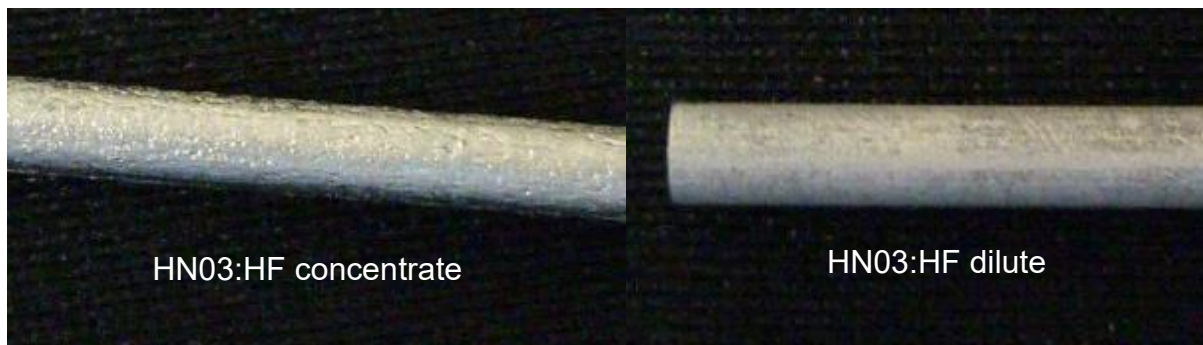
Figure 3-47 HF etching trial Ti tube sample results [114]
