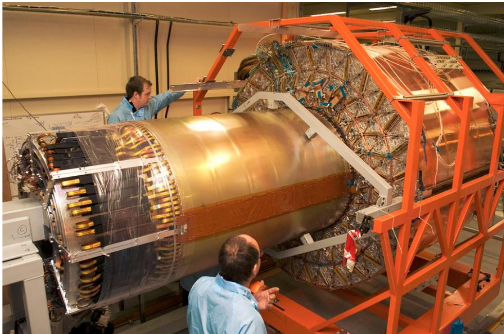
Figure 2-28 Image of TRT being integrated into the SCT Barrel [40]
