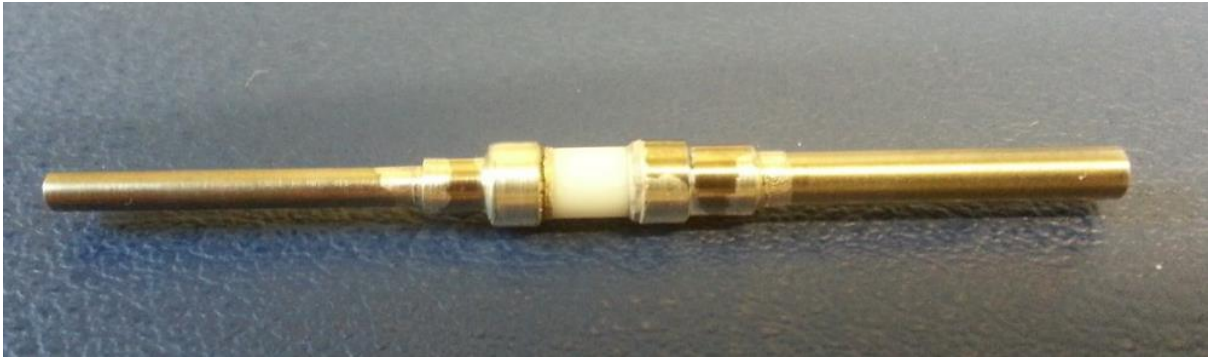
Figure 3-52 Image of prototype ITk Strip electrical isolator [97]
