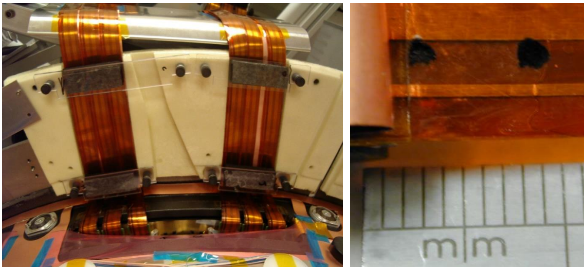
Figure 2-20 Photo of LMT testing (left) and failure (right) [30]
