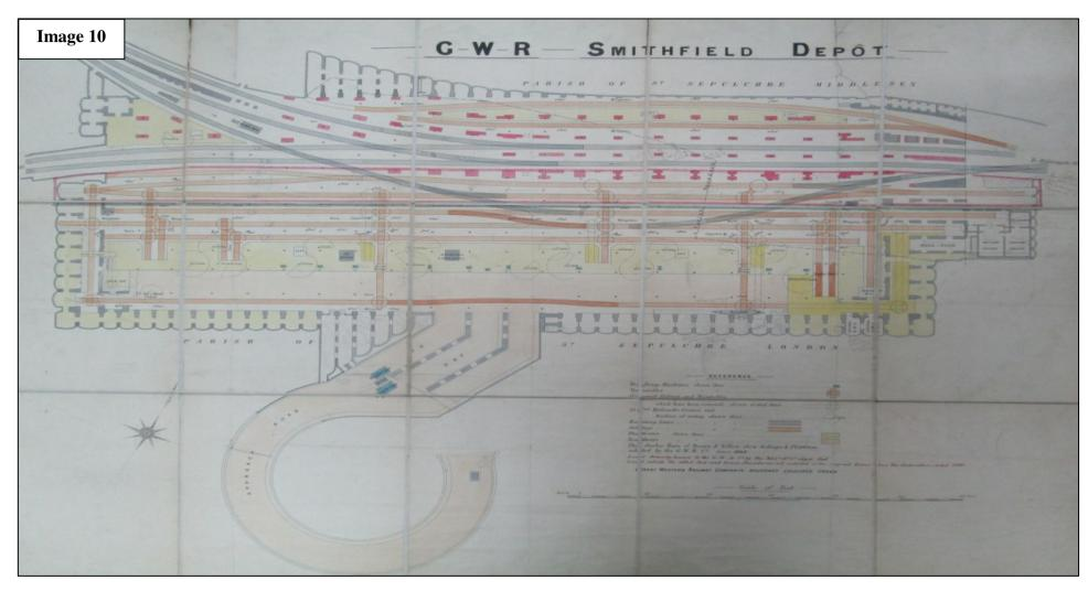
A 1912 colour plan of the GWR goods depot beneath Smithfield Market, central London with proposed alterations. Note the curved road ramp and the circles denoting turntables for shunting wagons in the confined space. Two lifts allowed meat to be directly conveyed to the market floor above. Source: TNA: RAIL 1030/213, 1912 Great Western way, 'Smithfield Station: C.G.M.O.'
