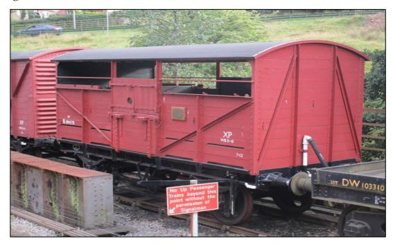
The basic features of the British Railways 8-ton cattle wagon, such as this example at the North Yorkshire Moors Railway had changed little from the standard Railway Clearing House design. Each wagon could be split into compartments with dividers. Note the apertures for draining effluent and the outside structural members on the wagon ends, so-designed to prevent injury to animals. Author's collection.
