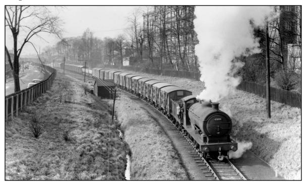
Ex-LNER J27 0-6-0 No. 65894 shunts BR PALVANS and coal hoppers outside Rowntree's Cocoa Works, Haxby Road, 1962. Note the works in the right background. The train is on the branch that linked the York-Scarborough line to the cattle market at Layerthorpe; the line also formed a connection with the independently-owned Derwent Valley Light Railway, the route of which served the arable district between York and Selby. Source: Kidderminster Railway Museum collection.
