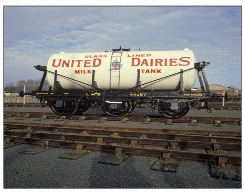
Restored LMS/United Dairies bulk milk tank No. 44057, which forms part of the National Collection of railway vehicles. This example is a later six-wheeled vehicle, built in 1937. Source: National Railway Museum NRM\_CT\_937988.
