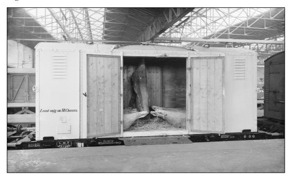
Beef loaded in an LMS "M-type" ventilated container, 1936. The carcases are protected by cloth sacking; also note the arrangement of carcases on the floor, a practice which allowed full utilisation of wagon capacity, yet shows little consideration for hygiene beyond straw bedding. Source: National Railway Museum 1997-7409\_LMS\_7990.
