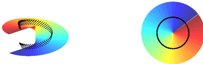
Figure 1.8: *A side on view with propagation upwards (left) and a top down view with propagation out of the page (right) of a vortex isophase surface. Colour represents distance along propagation and arrows show the local surface normal vector.*
