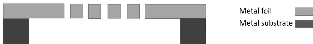
Figure 5.1: *A schematic cross section through the Pt foil amplitude mask. In this experiment the foil was  $1\mu\text{m}$  thick.*
