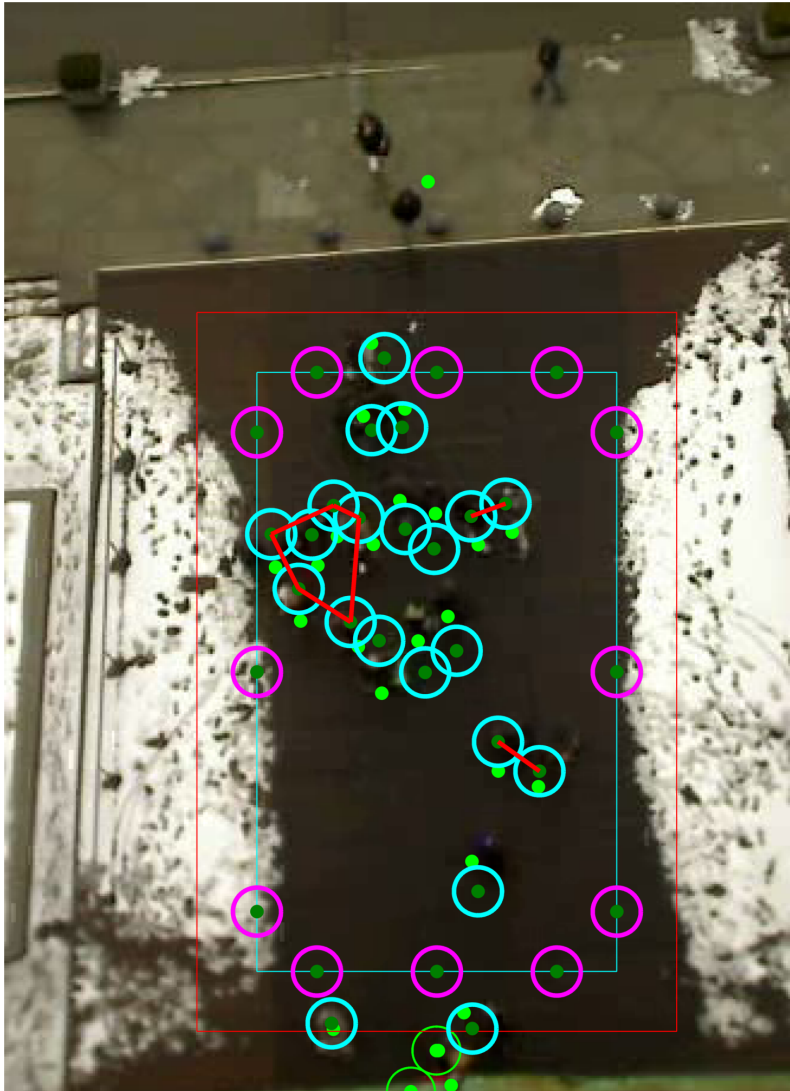
Fig. 7.3 Demonstration of how video frames that fulfil the requirements of the pedestrian scenarios are obtained. Pedestrians are represented by sky blue circles inside, and green circles outside of the red box, respectively. For a frame to be selected, the appropriate pedestrians must be within the red box, and also not intersect with any purple circles that represent any of the robot's start positions. The green dots in front of each pedestrian is its position in the next frame, used to calculate the pedestrians' velocities. The red convex polygon over the pedestrians represents a group of six pedestrians, and the two red lines indicate two couples moving together.
