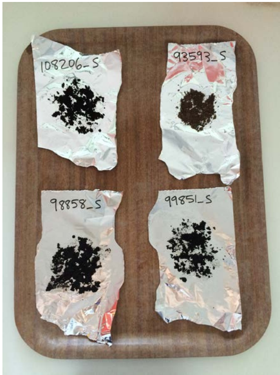
Figure AM4.1. Air drying soil samples.
