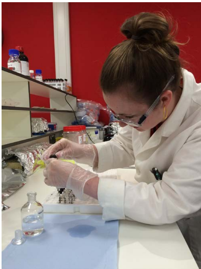
Figure AM4.4. Transferring aliquots of extracted residue samples to autosampling vials.
