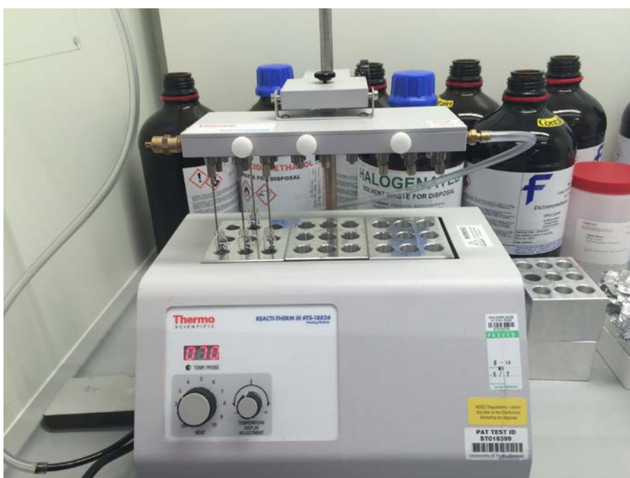
Figure AM4.3. Samples being evaporated under a stream of nitrogen while being heated at 70 °C.
