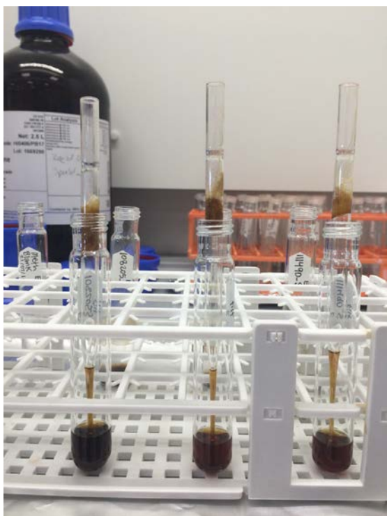
Figure AM4.2. Filtering soil samples through sterile glass wool.
