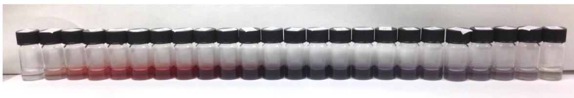
Figure 91: Photograph of sample vials of Sal-5-LICAM: iron(III) with highest ligand concentration to lowest ligand concentration from left to right, and highest iron(III) concentration to lowest iron(III) from right to left.
