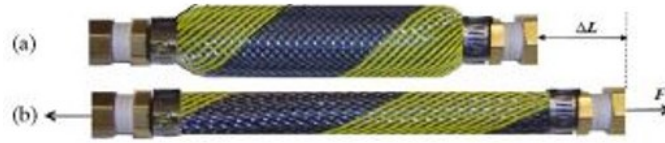
Figure 3.6: Diagram of McKibbens pneumatic muscle. (a) Relaxed muscle. (b) Actuated muscle [35].
