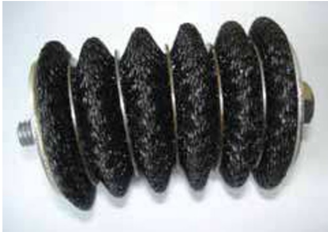
Figure 3.3: A pneumatic bellow [41]. Each ridge is called a convolute or whorl, with the wider ridges being called the outer convolutes and the narrower ridges being called the inner convolutes.
