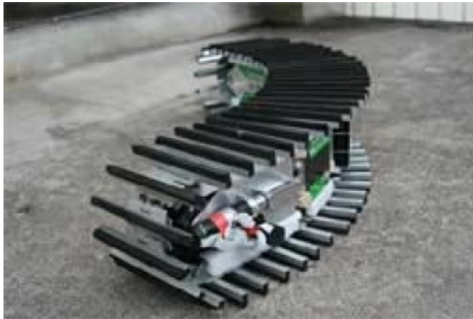
Figure 2.12: WORMY features 1 single track that is positioned round the whole robot to avoid it becoming beached [50].
