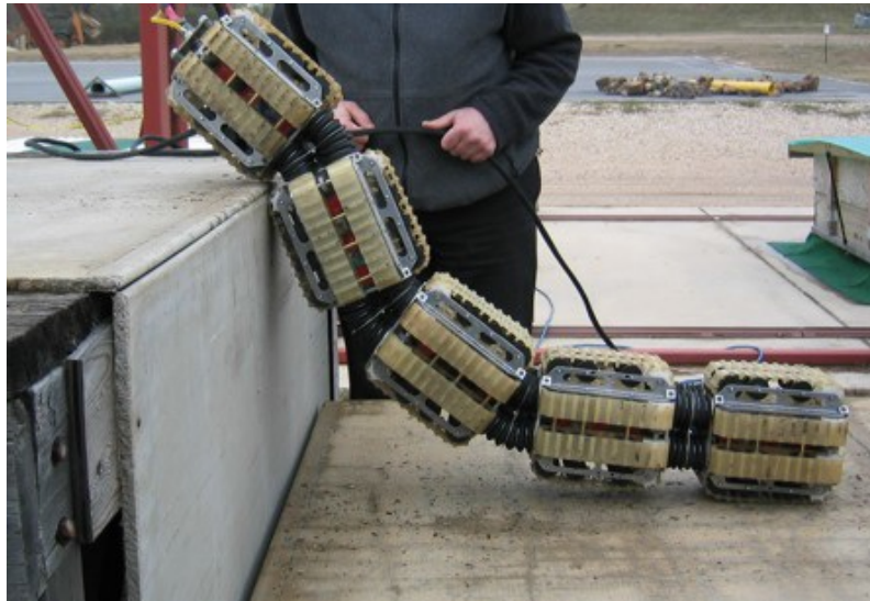
Figure 2.11: OT-4 controls its joint movement via four bellows per joint, which are flat when unactuated to save space and to reduce the risk of them becoming caught on foreign objects [42].
