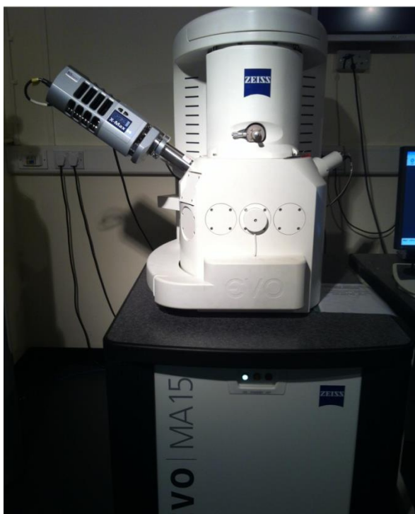
Figure 3.8 Photograph of SEM (Carl Zeiss EVO MA15) coupled with EDX (Oxford Instruments AZtecEnergy).
