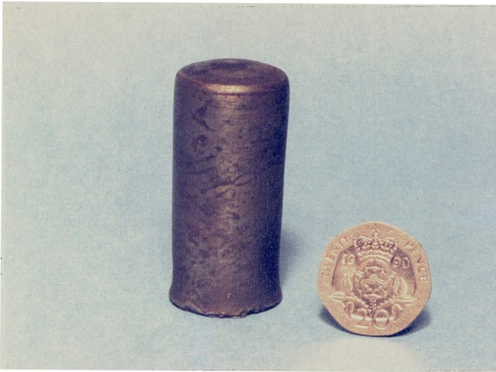
Fig. 1.18 Isostatically pressed sample of sintered NdFeB (Philips Components RES300).
