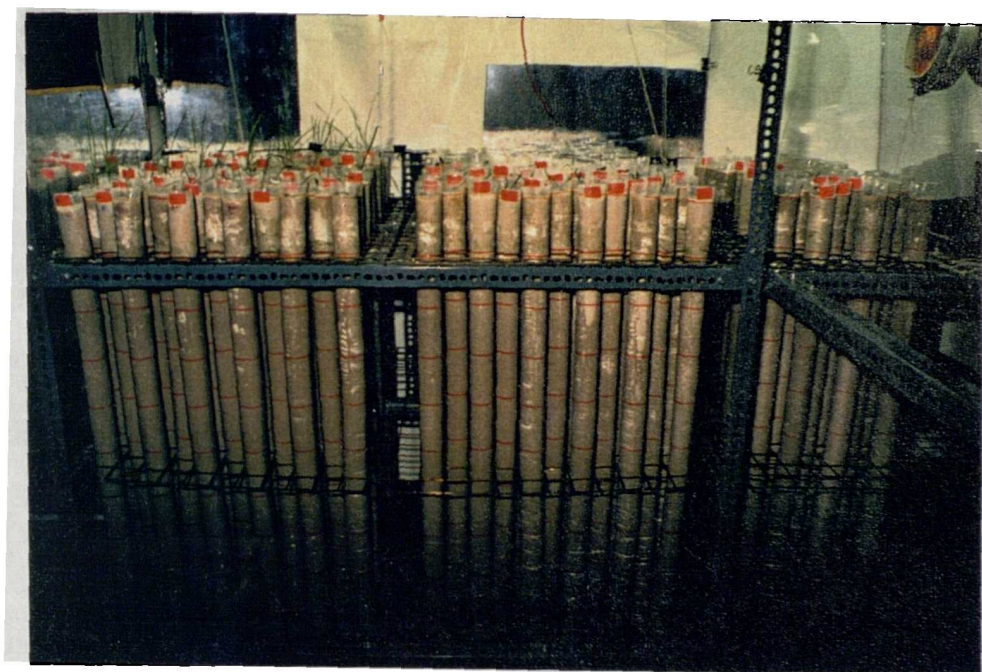
Plate 5.1: Side view of experiment with front reflecting panel removed to show the vertical tubes of sand.
