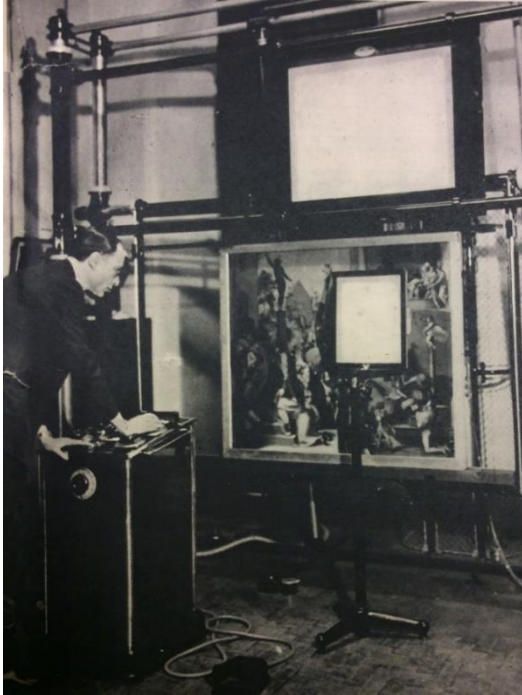
Figure 64. Photograph of The Illustrated London News , 4 th October 1947, showing a photographic reproduction of the Scientific Adviser, Ian Rawlins, taking an x-ray of one of the Gallery's pictures, British Library, London.
