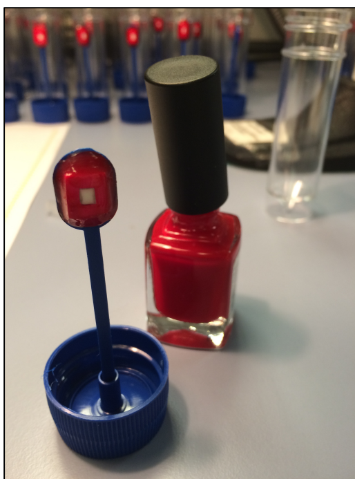
Figure 3-4: Application of nail varnish coating with exposed enamel window
