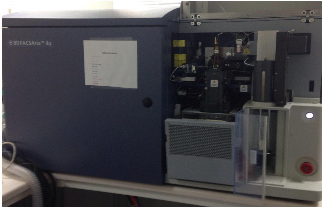
Figure 2.9 BD FACS Aria for sorting of mutant cells
