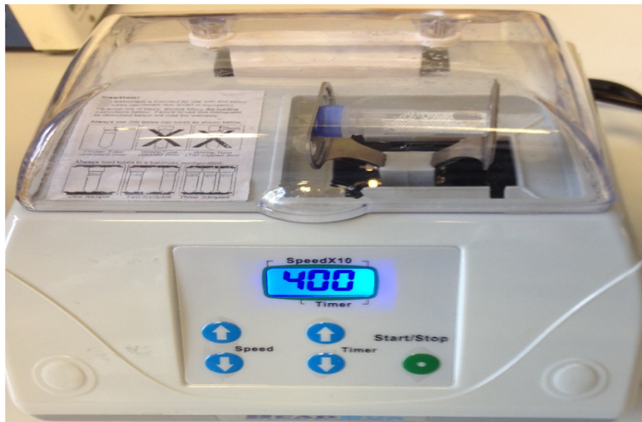
Figure 2.3 Bead bug microtube homogenizer for disruption of algal cells
