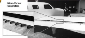
Enlarged area shows Micro VGs installed on the Rap of a Piper Malibu Meridian.
