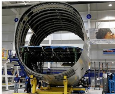
Figure 2.16: Left: Safe-life example of B787-10 body construction (Source: Ostrower, 2014). Right: A fail-safe example of reactor control rods (Source: Thuma, 2010)
