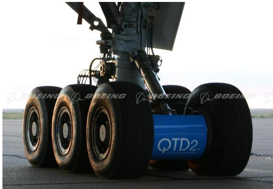
Quiet Technology Demonstrator Two (QTD2) Tobbogan fairings attached to MLG of B777 aircraft (source: www.boeingimages.com )
