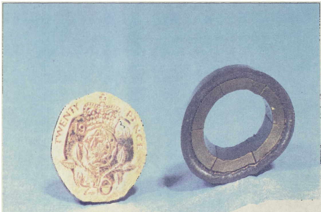
Fig 6.14 Photograph of the magnet segments used in the prototype actuator.
