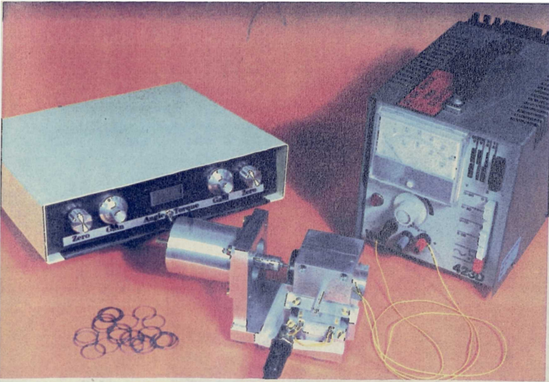
Fig 5.33 Experimental test rig for drag torque measurements.
