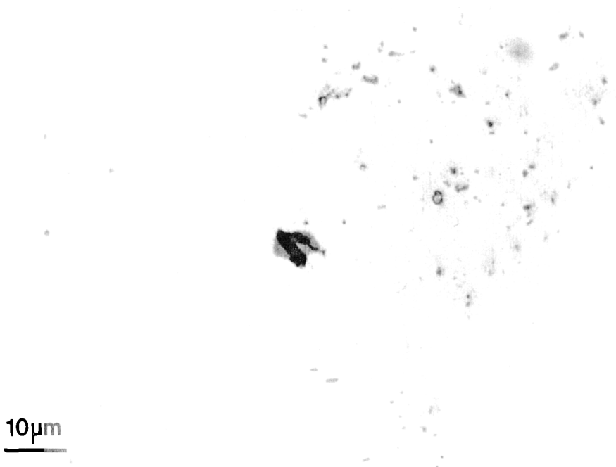
Figure 3.5 (a) Duplex type inclusion. grey: Manganese sulphide (MnS); Dark: Iron oxide (FeO).
