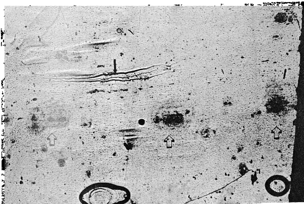
Figure 4.6(b) Stage I crack initiation from pits after 10000 cycles. N/N_f = 0.13 .
