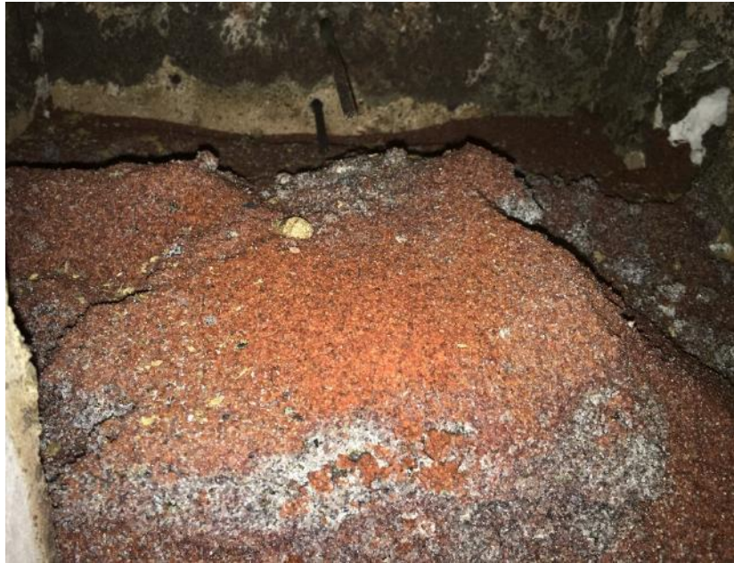
Figure 7-45 Agglomerated bed as a result of combusting straw pellets
