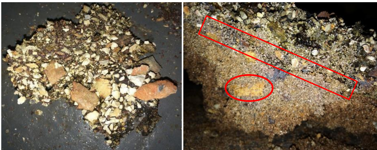
Figure 6-35 Images of agglomerates from the combustion of Pakistani coal with varying coal: limestone ratios. Left image showing the embedding of limestone in agglomerate, right image showing larger particles trapped in bed agglomerate with sintered top layer
