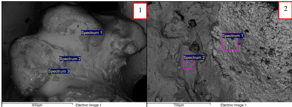
Figure 6-25 SEM images and the locations of SEM-EDX from wood combustion. Images are as follows; 1) agglomerated bed particles, and, 2) fusion point between limestone and bed particle
