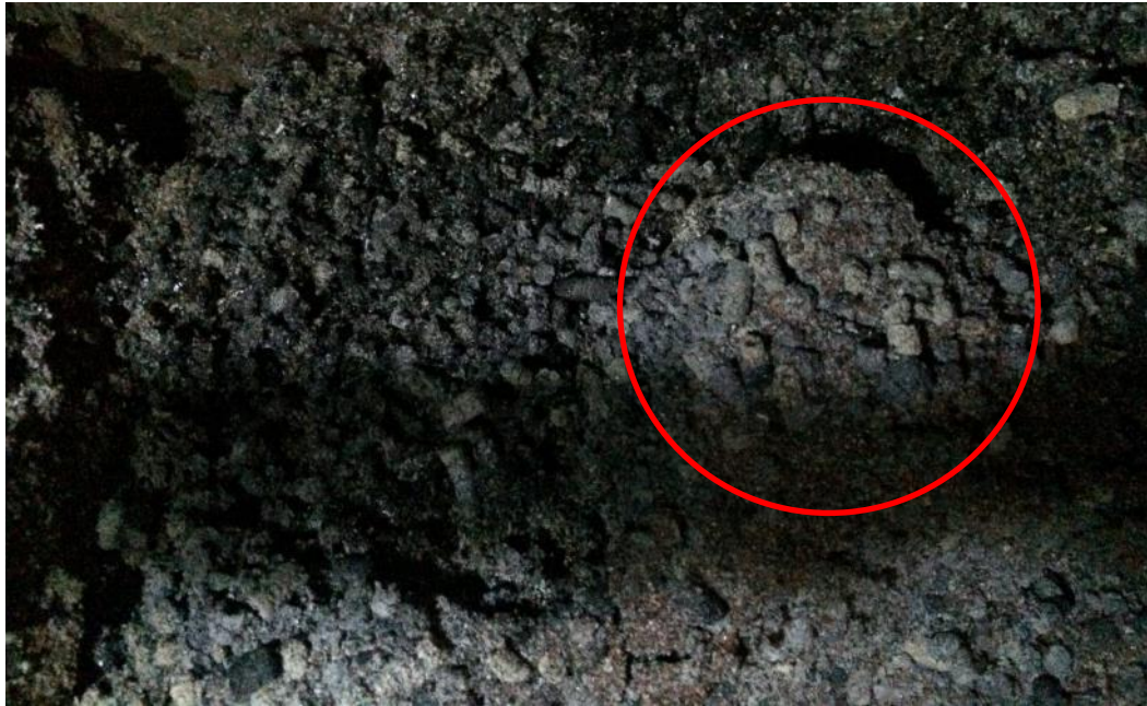
Figure 6-29 agglomerated structures and ashed pellets from the Co-firing of wood pellets and coal
