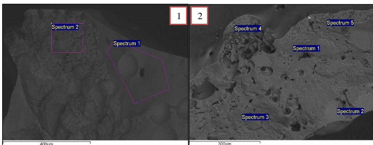
Figure 7-12 SEM images and location of SEM-EDX measurements from oats combustion. The images show the following; 1) cross section of agglomerate, and, 2) cross section of liquid agglomerate/sintered area
