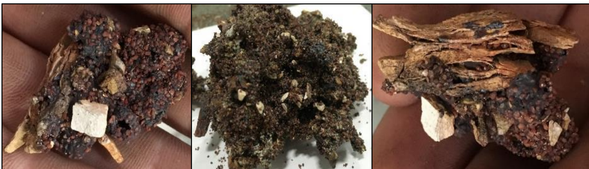
Figure 6-4 Agglomerates taken from the defluidised bed post testing of steady state combustion with Coal A
