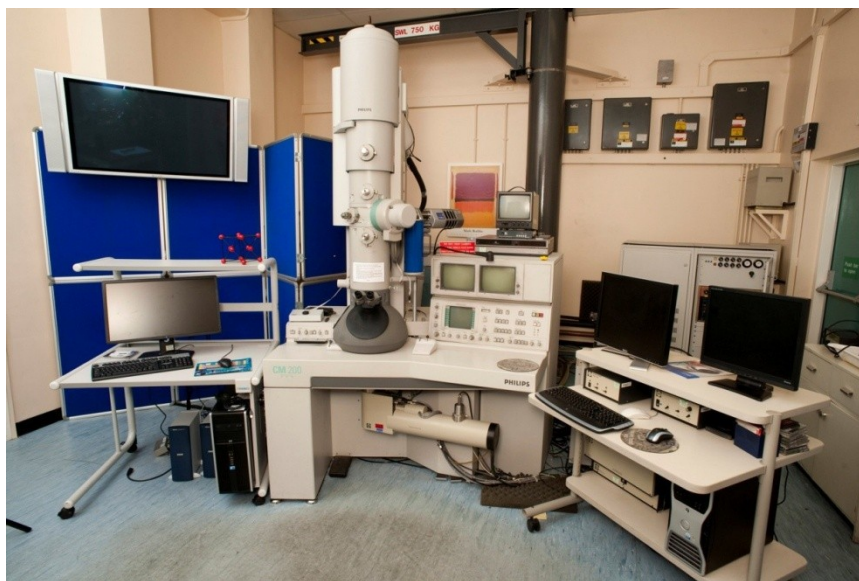
Figure 3.16 The Philips CM200 transmission electron microscope housed at the University of Leeds, UK.
