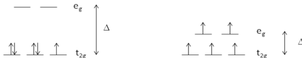
Figure 2.1 Electronic configurations of iron in low-spin (left) and high-spin (right) complexes with 5 d electrons.
