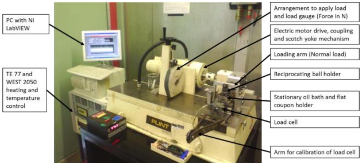
Figure 5-1: Annotated image of the Phoenix Plint TE 77 HFRR tribometer
