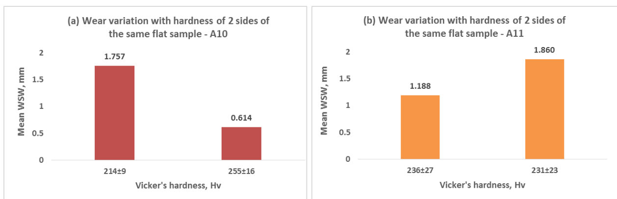
Figure 5-13: Wear variation with hardness of the two sides of flat samples (a) A10 and (b) A11.
