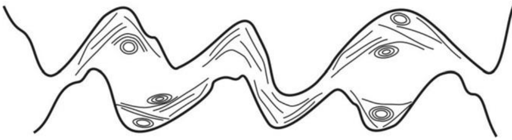
Figure 4-3: Model showing NP entry into the valleys on the contacting surfaces. Valleys on the surface (profile) act as reservoirs and help to preserve the NPs within the contact [110].
