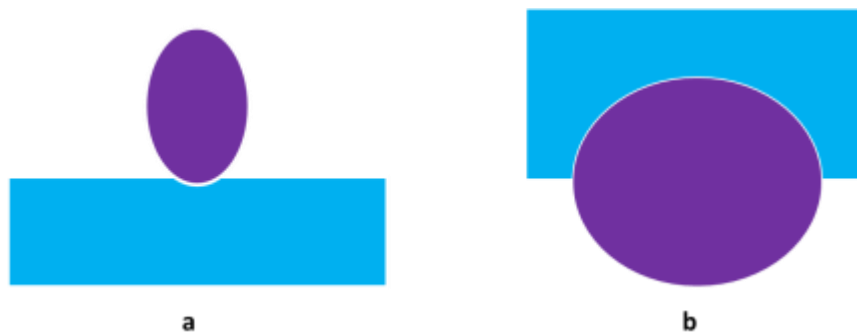
Figure 3-2: Tribological contacts (a) Non-conformal and (b) Conformal.
