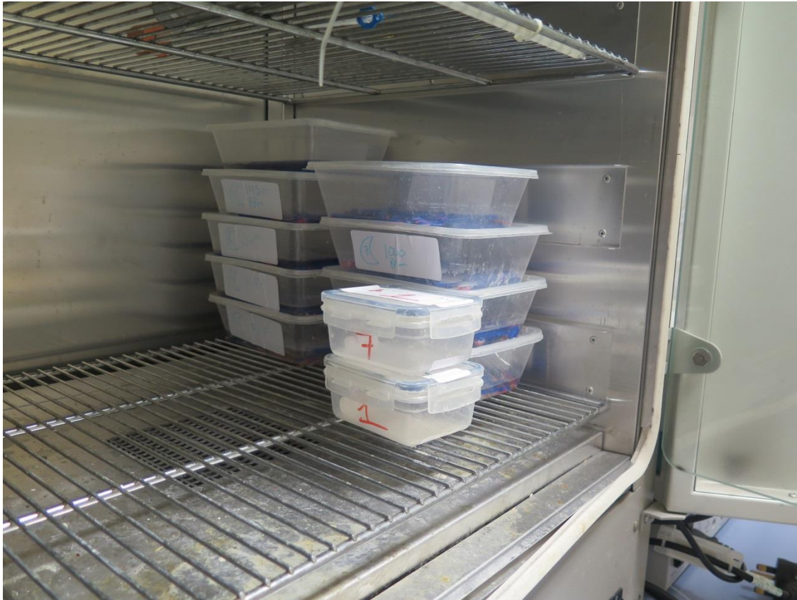
Figure 19 Enamel slabs were kept in incubator at 37°C at all times except during the dipping in the toothpaste slurry or the demineralisation solution
