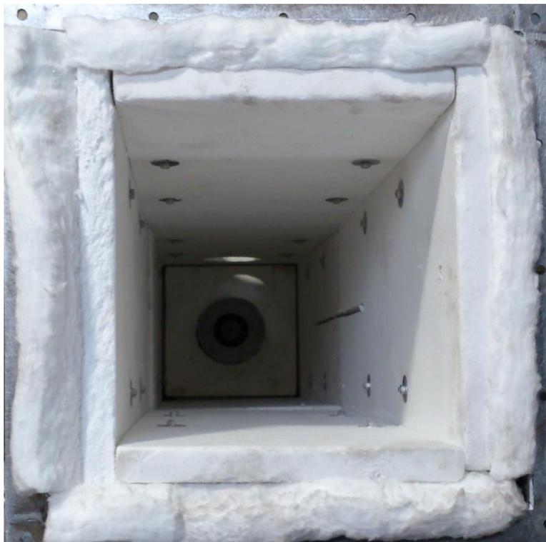
Figure 3-4 Photograph of the internal insulation of the utilised chamber.
