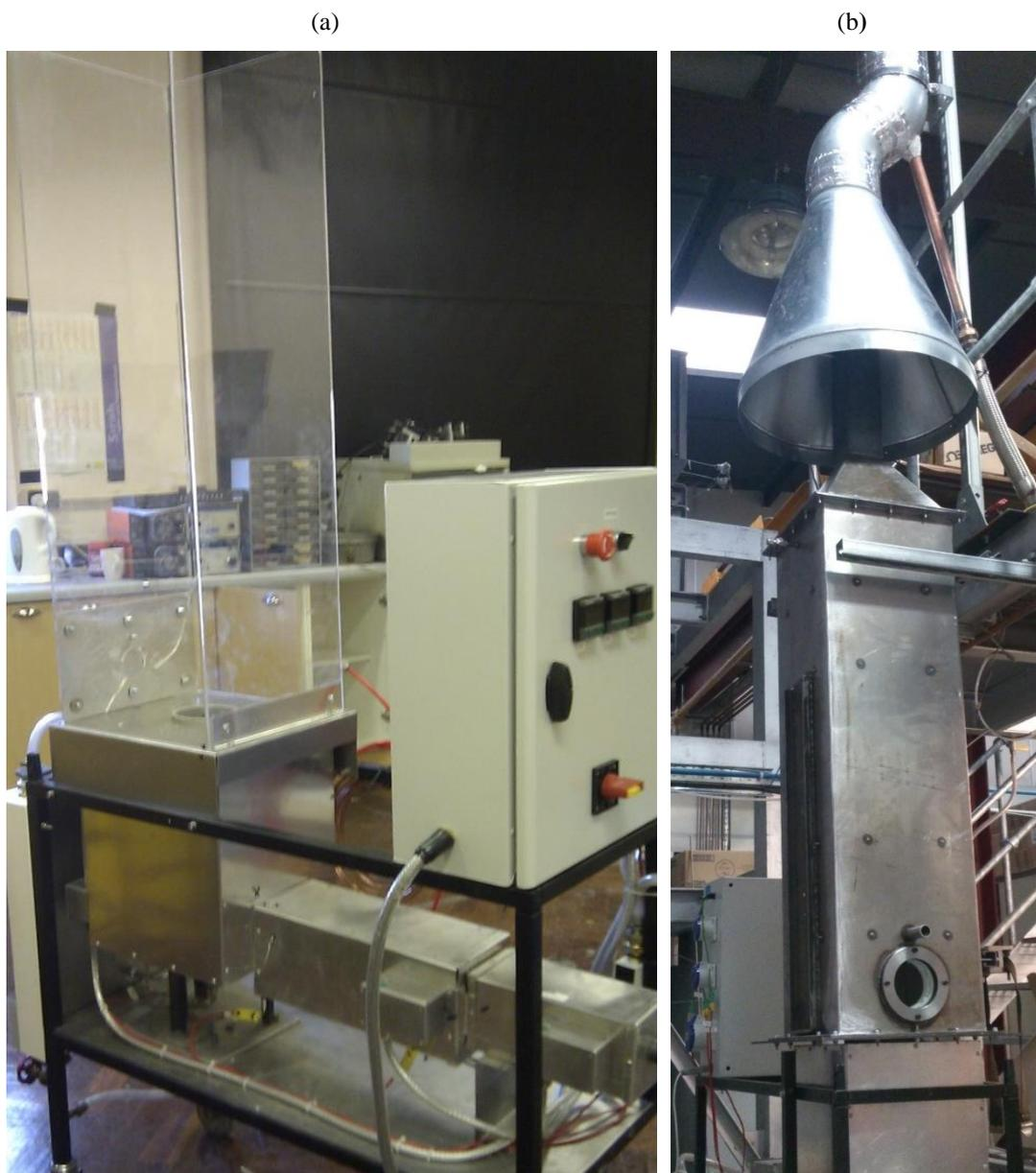
Figure 3-1 Photographs of the (a) old and (b) the modified combustion chamber.
