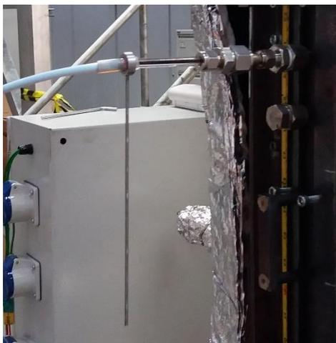
Figure 3-13 Photograph of the probe alignment procedure using a pointer.
