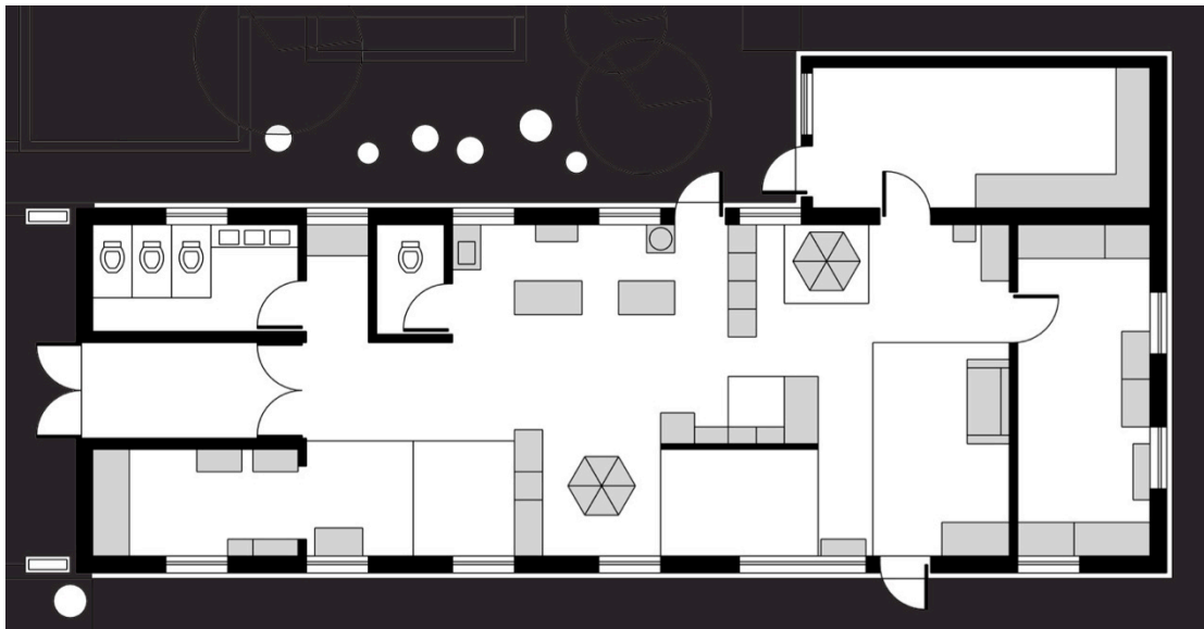
Figure 10: Plan of the single storey annexe playroom building
