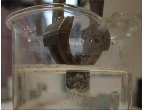
Figure 86. A photograph taken during the dissolution of the  $\text{NaAlO}_2$  preform
