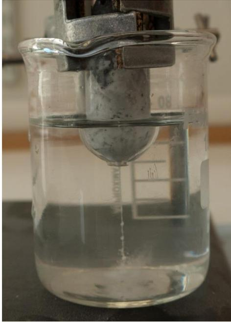
Figure 76. A photograph of in-crucible dissolution of  $\text{NaAlO}_2$ .
