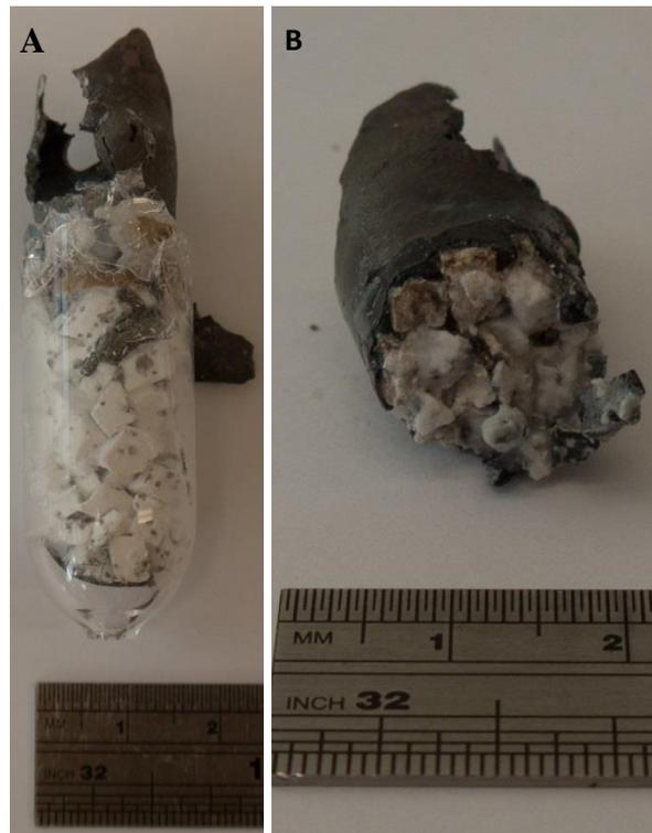
Figure 80. (A) A Photograph of infiltrated Ti-811 alloy while still in a quartz crucible pre heat treatment (B) Post heat treatment and removed from the quartz crucible
