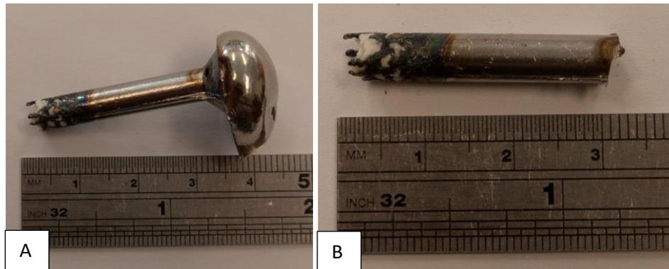
Figure 63. A photograph of the first replication casting iteration. Sodium aluminate can clearly be seen on the left of the casting. (A) with the residual Ti-811 in place. (B) with the residual alloy removed.
