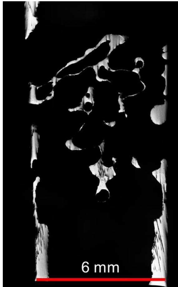
Figure 66. An optical image of a cross section of the replication casting.
