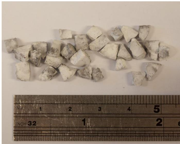
Figure 29.  $\text{NaAlO}_2$  particles prepared for use in production of a larger pore size foam. The particles shown have been through a casting cycle, but were then recovered as they were located at the bottom of the crucible and not reached by the metal.
