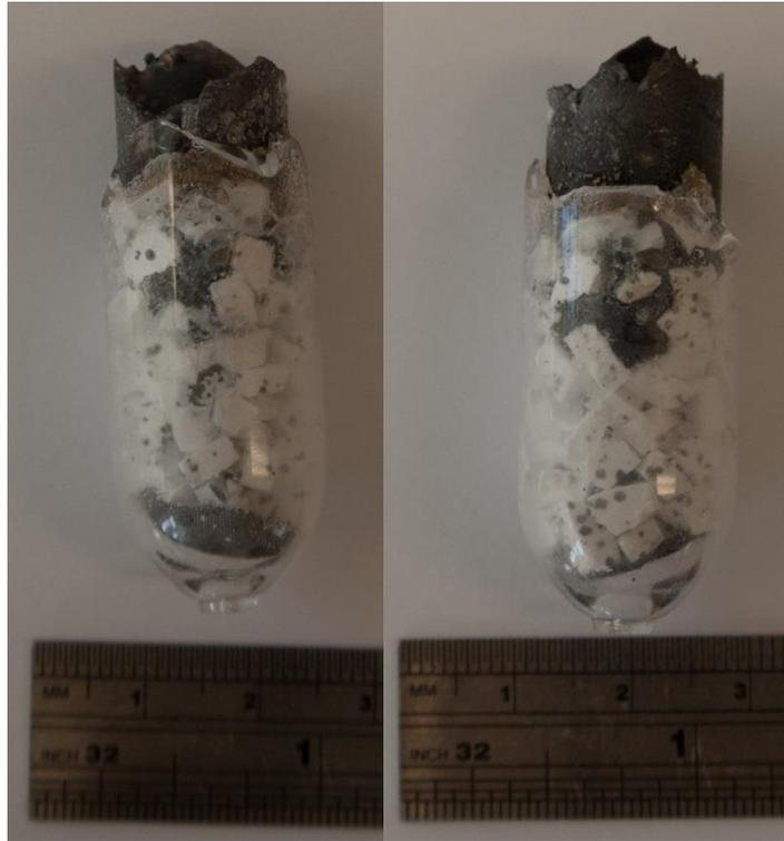
Figure 75. Two photographs of the large particle continuous argon infiltration which show tendrils of alloy in at least two locations
