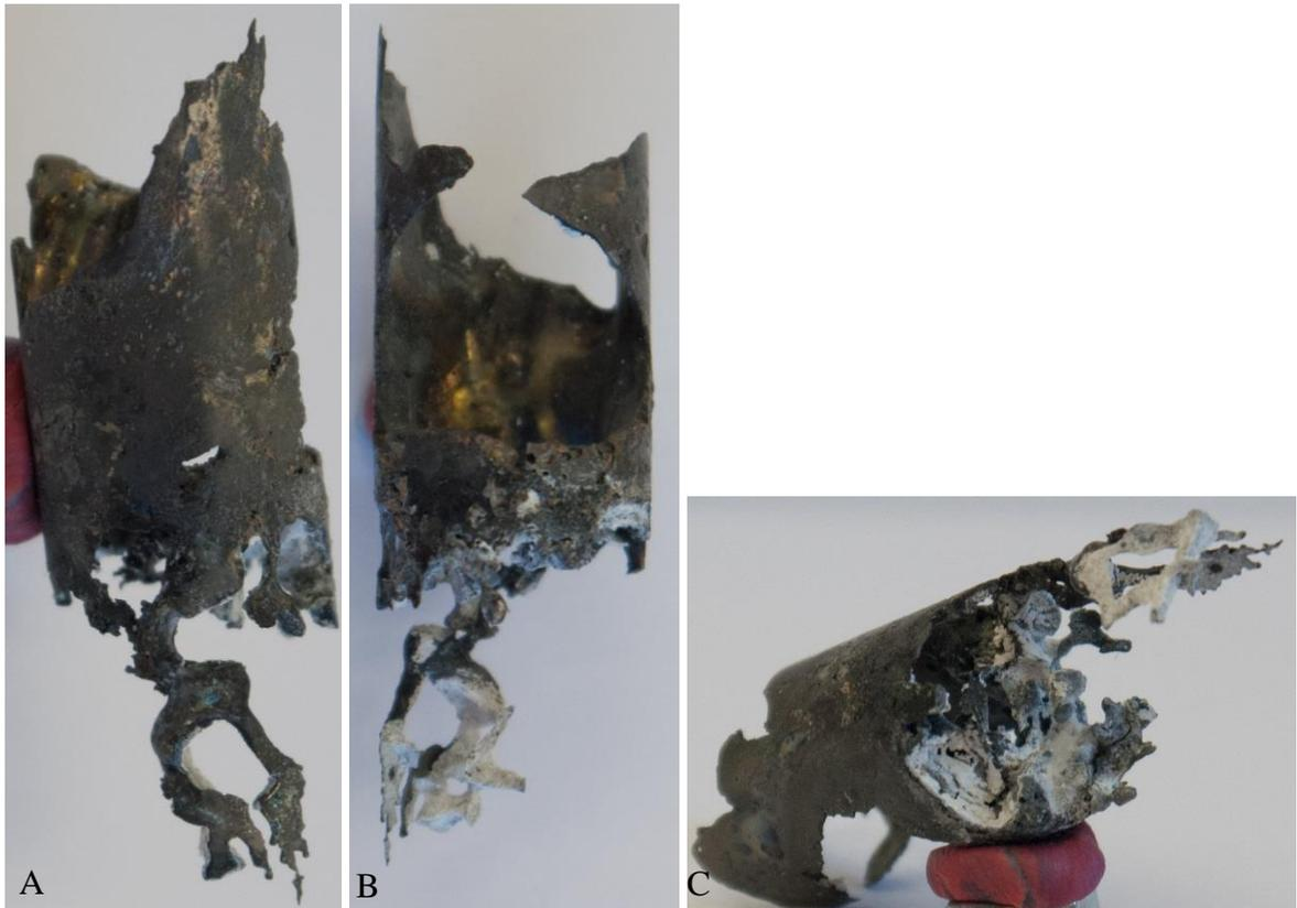
Figure 88. (A) A photograph of an infiltration cast with long tendrils of alloy. (B) An alternative view of the infiltration. (C) A photograph of the central pore network that formed
