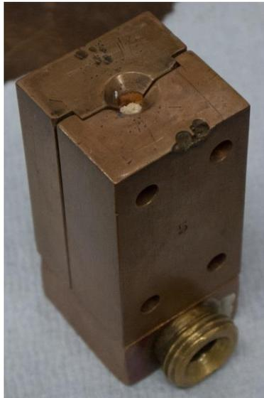
Figure 67. A photograph of the copper mould ready to be placed into the arc melter, with the  $\text{NaAlO}_2$  visible at the top of the opening
