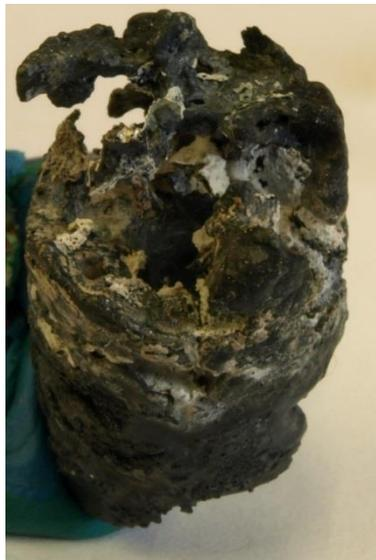
Figure 87. A photograph taken of the infiltration cast Ti-811 after  $\text{NaAlO}_2$  removal
