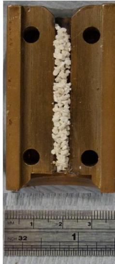
Figure 68. A photograph of the copper mould after casting with NaAlO<sub>2</sub> still in-situ showing zero infiltration.
