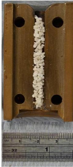
Figure 28. Cross section of the mould assembly with the sodium aluminate in-situ.
