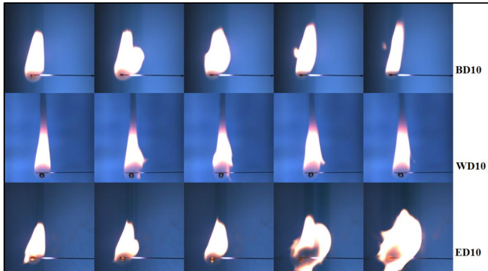
Figure 4-22: The effect of puffing on the shape of the flame surrounding the burning multicomponent fuel droplets.
