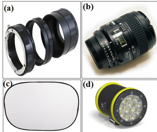
Figure 3-11: Components of the optical setup used for backlit imaging of the droplet combustion: (a) Extension tube, (b) Lens, (c) Light diffuser, (d) Light source.
