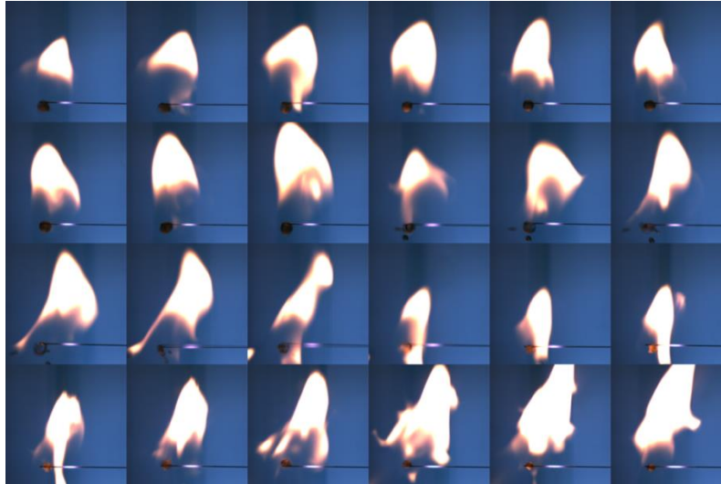
Figure 4-23: The effect of droplet microexplosion on the shape of the flame surrounding an ED10 fuel droplet.
