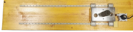
Figure 2.2: The bespoke 3D printed manipulandum used throughout this thesis. Its displacement along the linear tracks could be measured via a linear potentiometer (depicted) or a high speed gaming mouse mounted under the handle.
