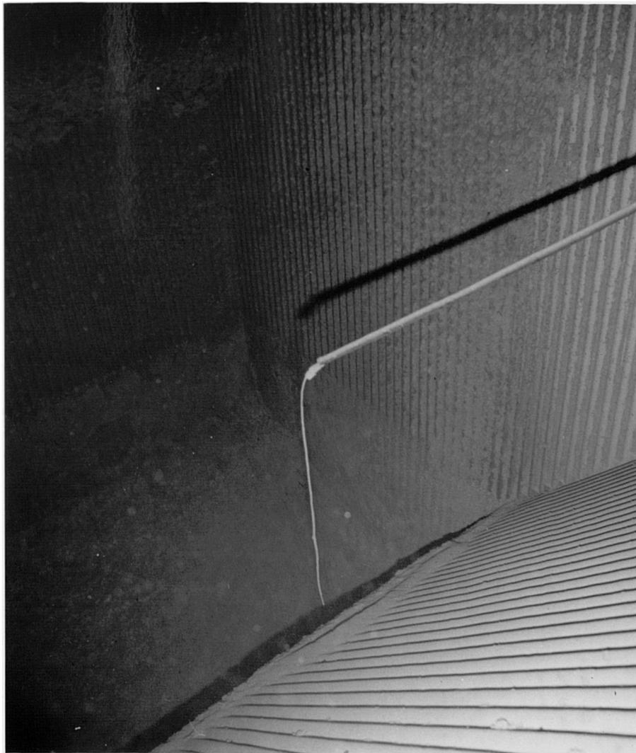
**PLATE 5 - End view of the water-cooled probe
