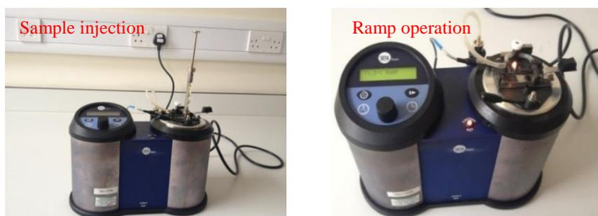
Figure 3.36 Setaflash closed cup equipment.
