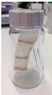
Figure 4-36. Passive sampling bag in a sealed vial.
