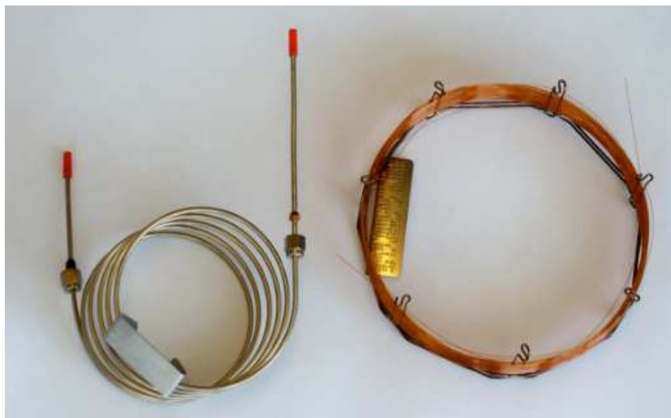
Figure 1-4. Left: Packed GC column; Right: Capillary GC column.
