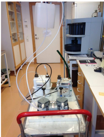
Figure 4-32. Active sampling set-up with pumps and volumetric flow meter.
