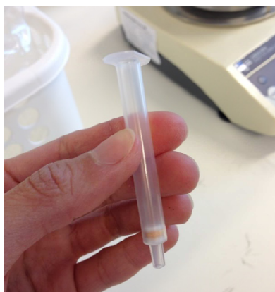
Figure 4-15. A ready 1 mL cartridge filled with 10 – 15 mg of ENV+ sorbent.
