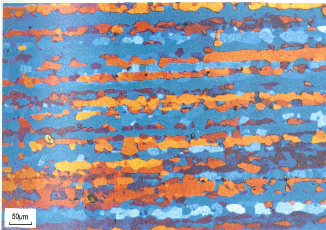
Figure 4.66(e) Optical micrograph of MONO material, rolled at 300°C and subsequently solution heat treated for 14 days.
