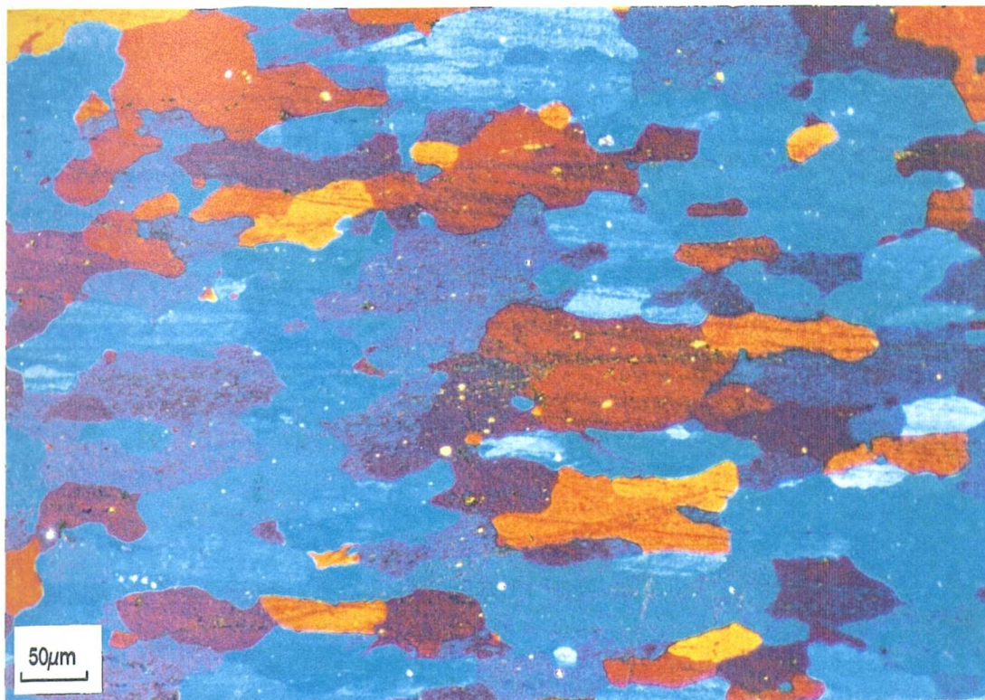
Figure 4.63(d) Optical micrograph of ASC material, rolled at 300°C and subsequently solution heat treated for 20 minutes.
