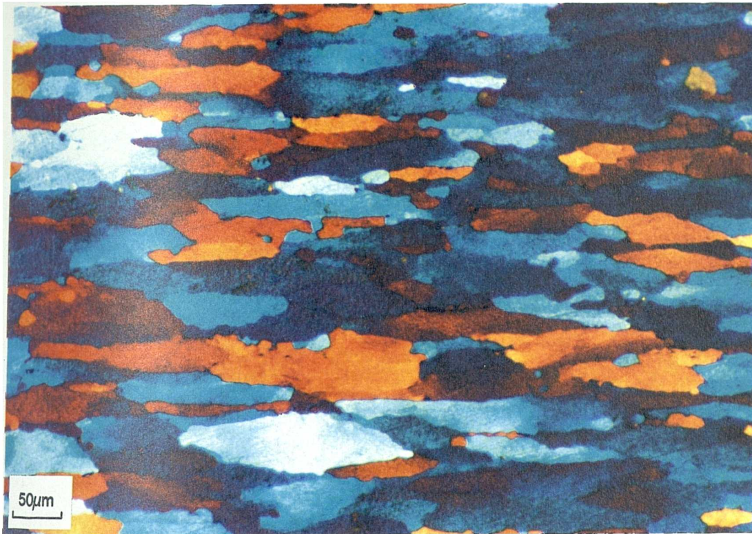
Figure 4.61(e) Optical micrograph of ASC material, rolled at 480°C and subsequently solution heat treated for 7 days.
