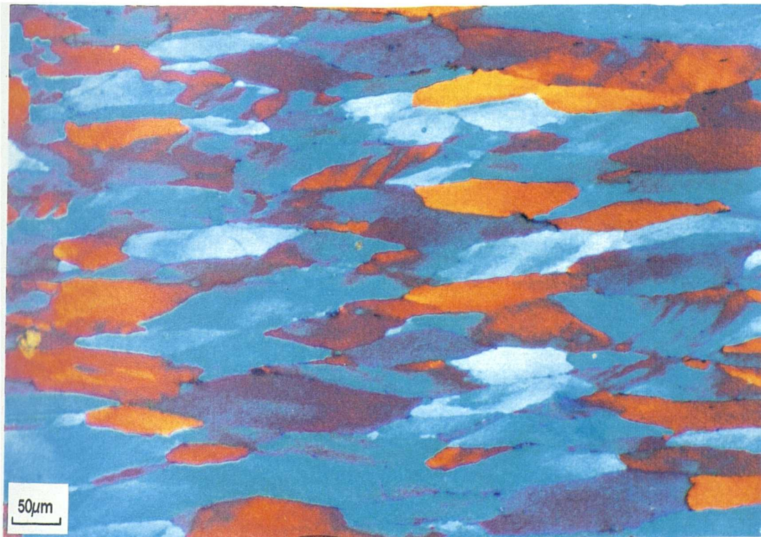
Figure 4.61(b) Optical micrograph of ASC material, rolled at 480°C and subsequently solution heat treated for 1 hour.
