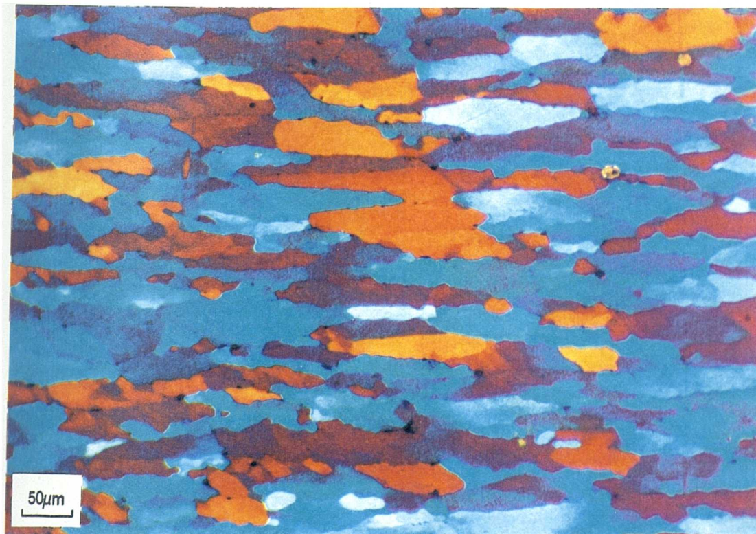
Figure 4.61(f) Optical micrograph of ASC material, rolled at 480°C and subsequently solution heat treated for 14 days.
