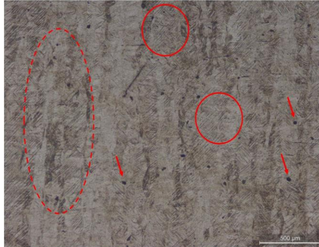
Figure 5-3 Sample E3 with martensitic \alpha' laths highlighted by solid lines, growing inside columnar prior \beta grains highlighted by the dashed line, with pores highlighted by arrows.
