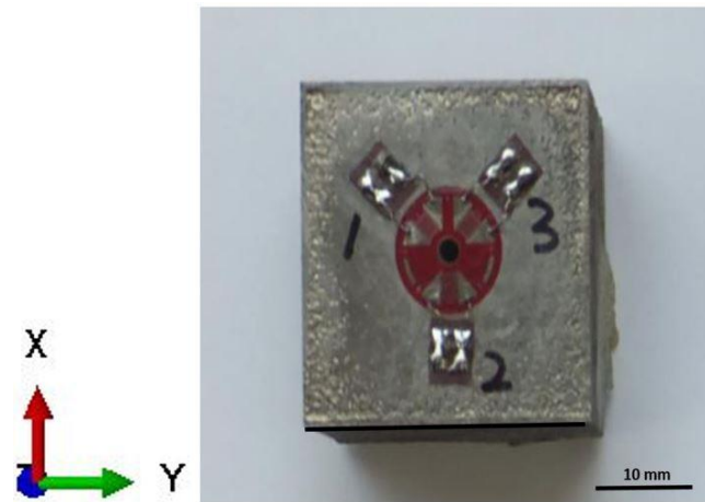
Figure 3-8 Residual stress specimen with strain gage rosette showing hole drilled in centre to measure residual stress on the top of the specimen in XY plan.
