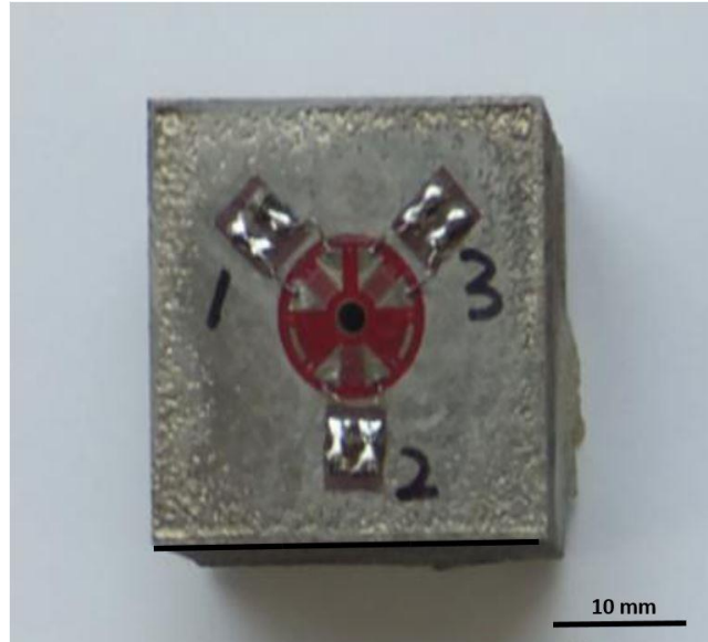
Figure 2-23 Residual stress specimen with strain gage rosette showing hole drilled in centre
