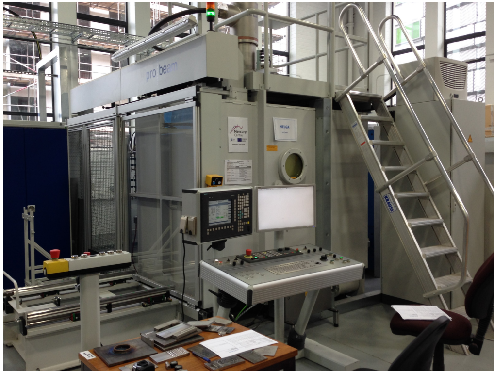
Figure 3.2 EBW (Probeam) machine.
