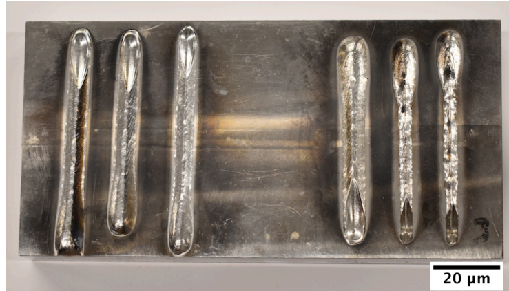
Figure 3.11 Beads on plate experiments of Ti6Al4V.
