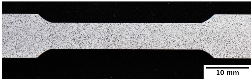
Figure 3.21 Macrograph of tensile test sample with speckle pattern prior to DIC test.
