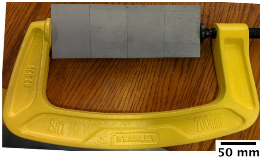
Figure 3.5 Fixture of the first butt welds.
