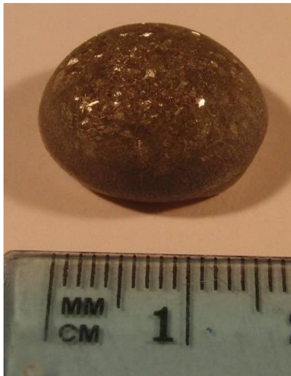
Figure 72. Example ingot of alloy GB1-AC produced using the Edmond Buehler arc melter.
