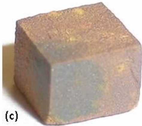
Figure 89. Alloy GB2-AC oxidised specimens. (a) GB2-AC-800-100h, (b) GB2-AC-1000-100h, (c) GB2-AC-1200-100h.
