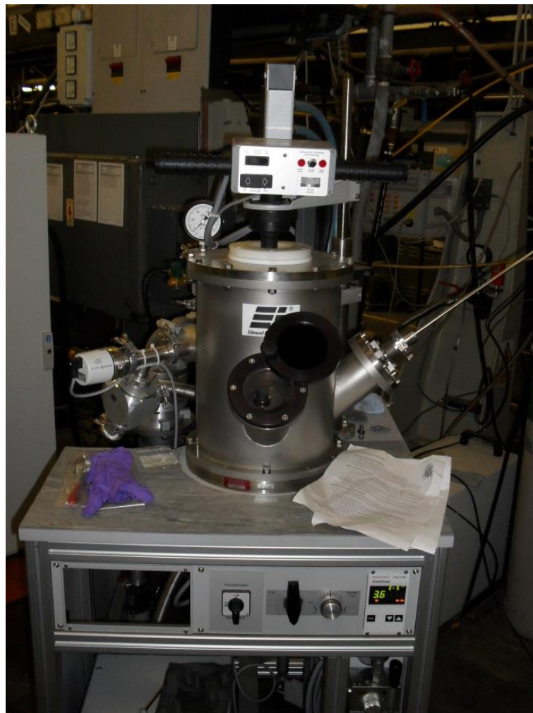
Figure 70. Edmond Buehler arc melter used for casting the GB1 and GB2 ingots. Courtesy of the Department of the Materials Science & Metallurgy of the University of Cambridge.
