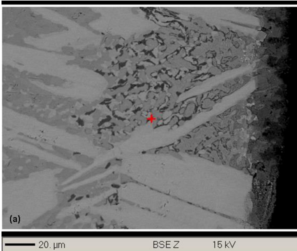
Figure 120. BSE image of GB1-HT oxidised at 1200°C for 50h.
