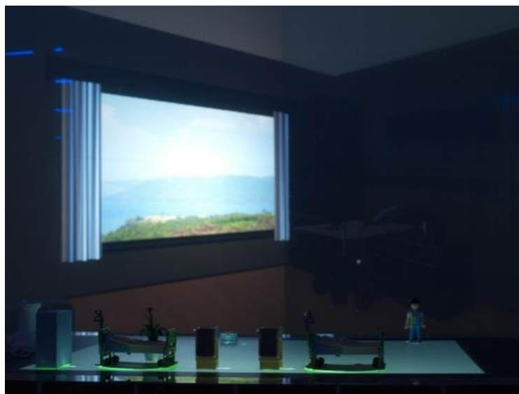
Figure 2.10 The Room Layout Configurator consists of a Surface Table with tangible objects which are connected to the virtual objects on the wall display.
