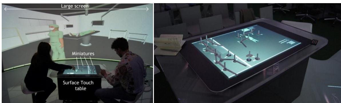
Figure 2.12 As shown in the right image, the Surface Table displays the floor plan of the Operating theatre and there are a set of miniature tangible CMA systems on top of it for supporting PD among stakeholders. The left image illustrates the user scenario of this MR application in which the platform in the right image is used an interface for the virtual theatre (shown in the background).
