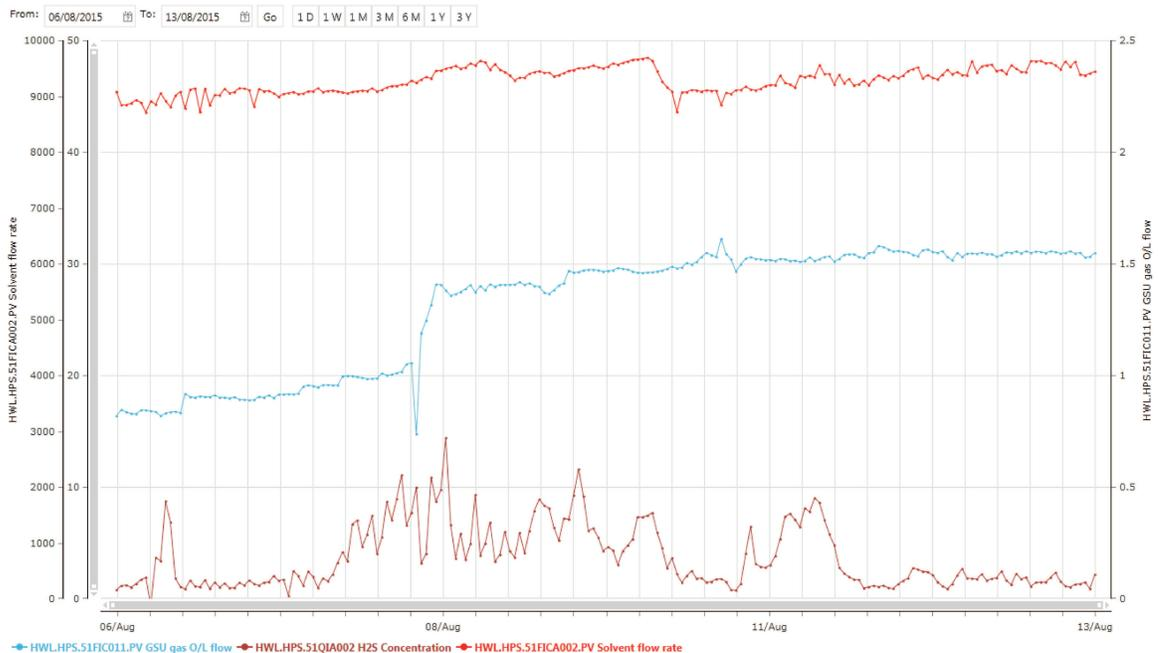
Figure C.1: PDO Harweel GSU. Blue: Gas flow rate (Range 0 - 2.5 MMSCMD), Brown: H<sub>2</sub>S concentration (Range 0 - 50 ppm), Red: Solvent flow rate (Range 0 - 10000 m<sup>3</sup>/d)
