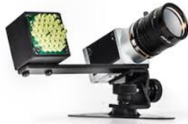
Figure 5-17 SmartEyePro camera and their position in the experiment room (Source: Rogue-Resolution, 2016). The SmartEyePro system consisted on two infrared cameras oriented towards the participant's face. This infrared cameras are able to detect the pupil in dark environments.
