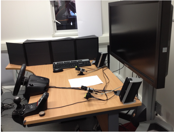
Figure 5-17 SmartEyePro camera and their position in the experiment room (Source: Rogue-Resolution, 2016). The SmartEyePro system consisted on two infrared cameras oriented towards the participant's face. This infrared cameras are able to detect the pupil in dark environments.
