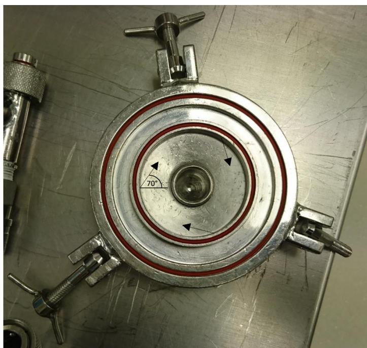
Figure 7.6: Grinding chamber of 2 inch Micronizer®
