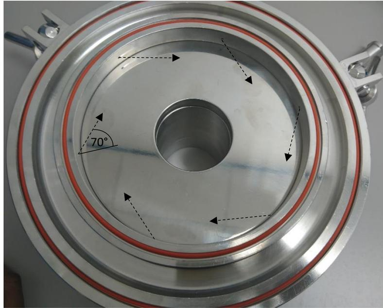
Figure 7.7: Grinding chamber of 4 inch Micronizer®
