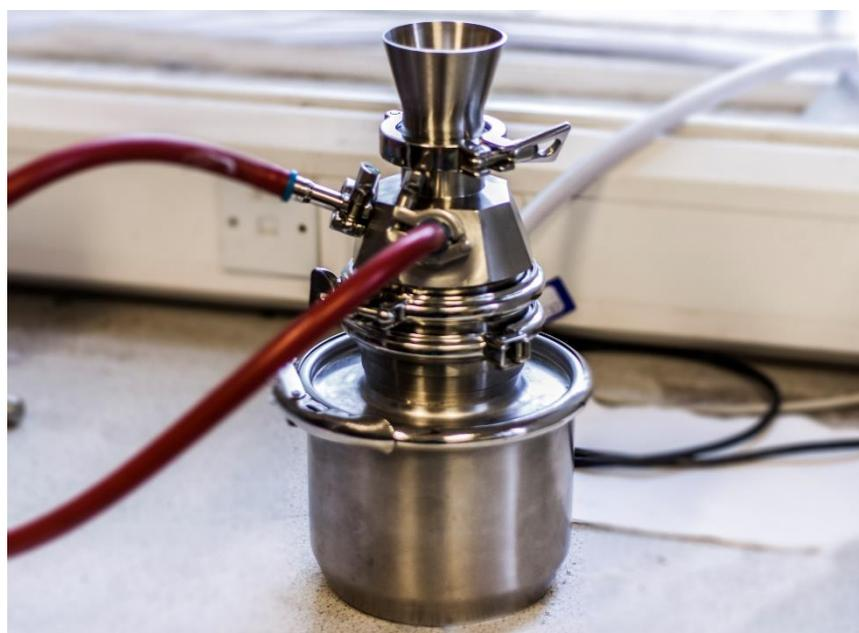
Figure 5.3: Hosokawa Aeroplex Spiral Jet Mill 50AS
