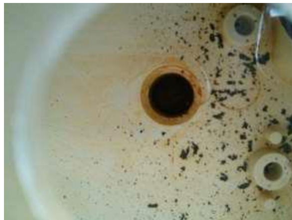
Figure 6.25: visual observation of AlCr(N) coating (spallation) after applied six successive DC/OCP cycles
