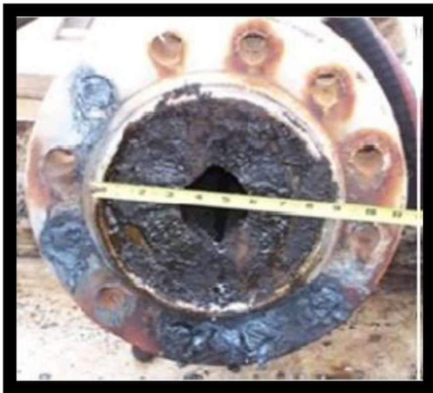
**Figure 1.2. Flowline clogged by scale [6].**
