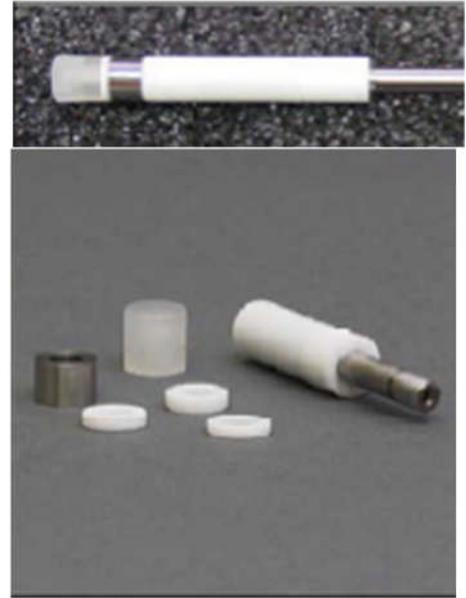
Figure 3.11a. Illustration of Rotating Cylinder Electrode (RCE) and its components.
