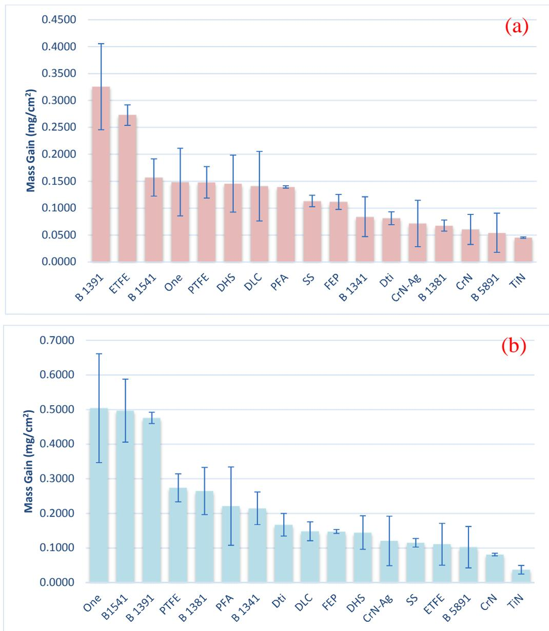
**Figure 5.2. Scale deposits thickness growth of different modified substrates in the *adhesion* tests, where the focus is on *adhesion* of pre-precipitated of scale crystals, in (a) laminar and (b) turbulent conditions.**
