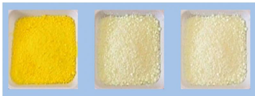
Figure 5: The colour differences between the photoinitiators used in resin based composites showing CQ (left), PPD (middle) and TPO (right), ( Bluephase LED user guide, Ivoclar Vivadent )
