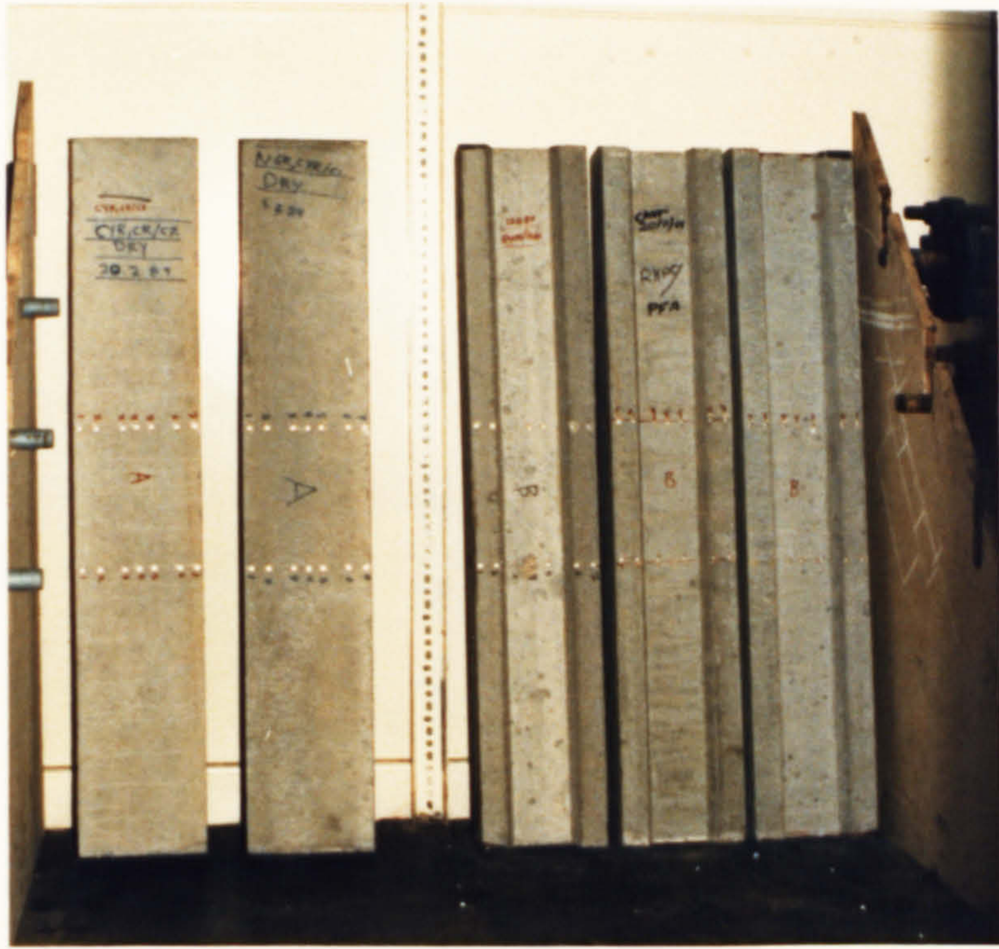
Plate 3.1 Control shrinkage rectangular and I-shaped beams placed in the vertical direction
