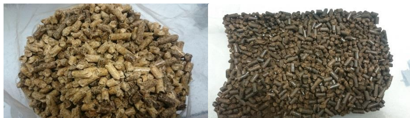
Figure 4.1: Biomass samples used in this work, North American white wood pellet (left) and torrefied spruce (right)
