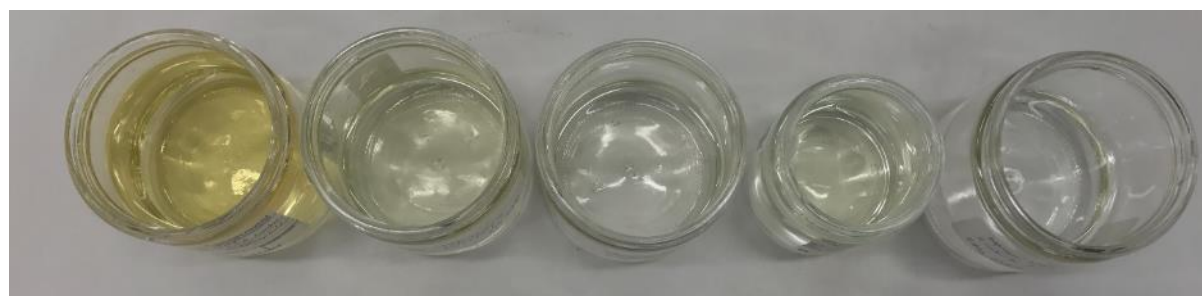
Figure 11-9. Photos of the impinger condensate for Wood A, pine, torrefied briquettes, peat briquettes and smokeless fuel (left to right).
