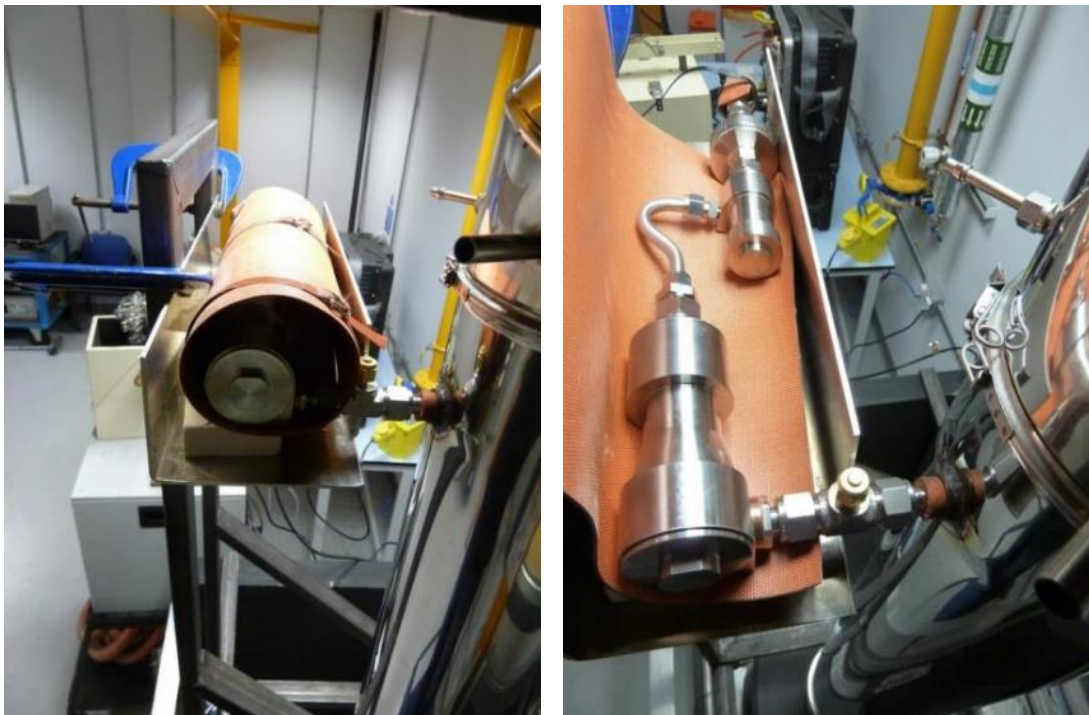
Figure 3-9. Images showing the setup of the cyclone separators and heating system.
