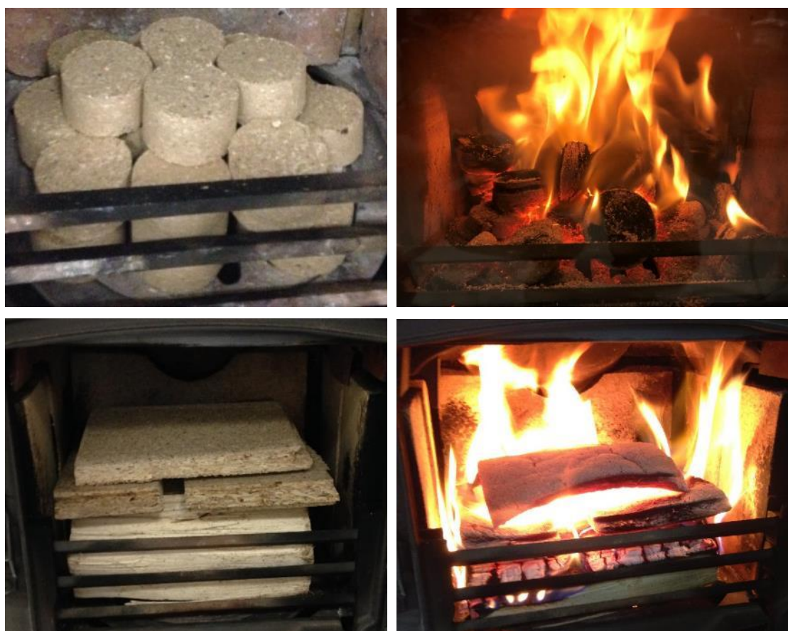
Figure 10-7. Photos of the waste wood emissions tests for (a) homogenised briquettes and (b) chipboard with fraxinus sp.
