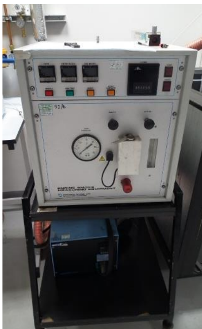
Figure 3-7. Smoke meter used in the tests.
