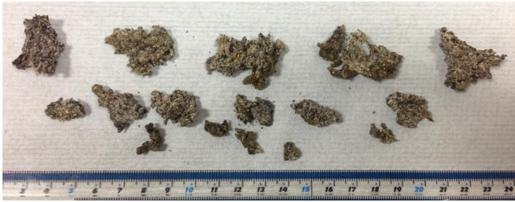
Figure 11-17. Photo showing clinker formed during the reed briquette combustion test.
