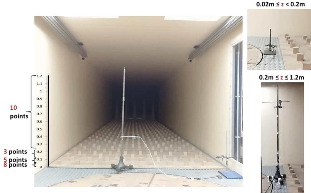
Figure 3-9 Illustration of location points for the velocity measurements in the roughness-line (left), along with the hot wire stands used per height case (right).
