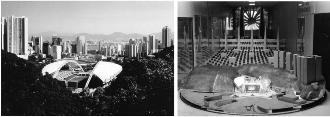
Figure 2-6 Illustration of the Hong Kong stadium structure (left) and 1:300 wind tunnel scaled model (right) (Thompson et al., 1998).
