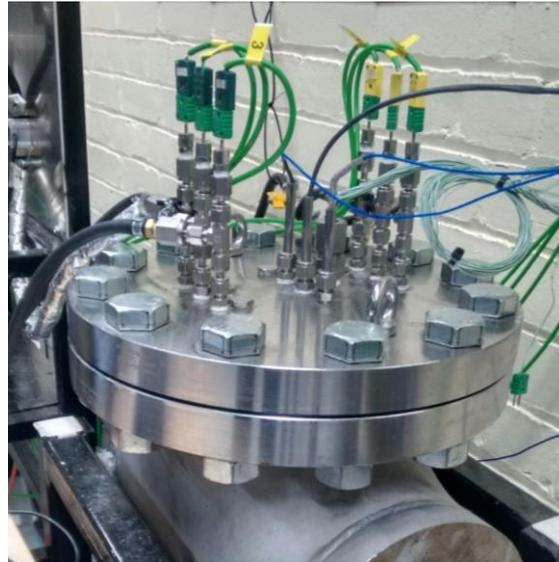
**Figure 3.14:** Cooling and heating connections for water temperature measurement
