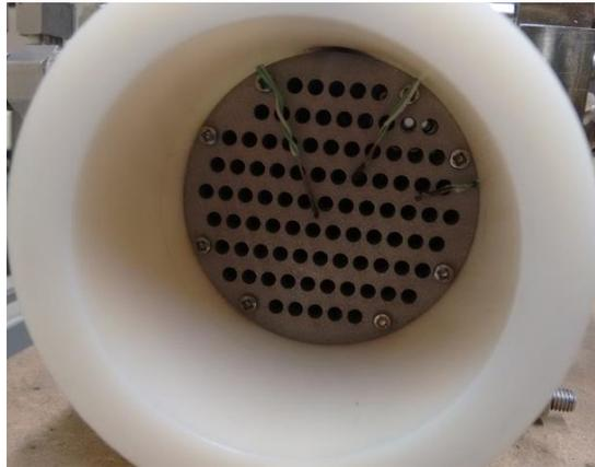
**Figure 3.6:** Arrangement of the thermocouples within the heat exchanger in the gas environment (dimensioned drawing is given in Appendix – E).
