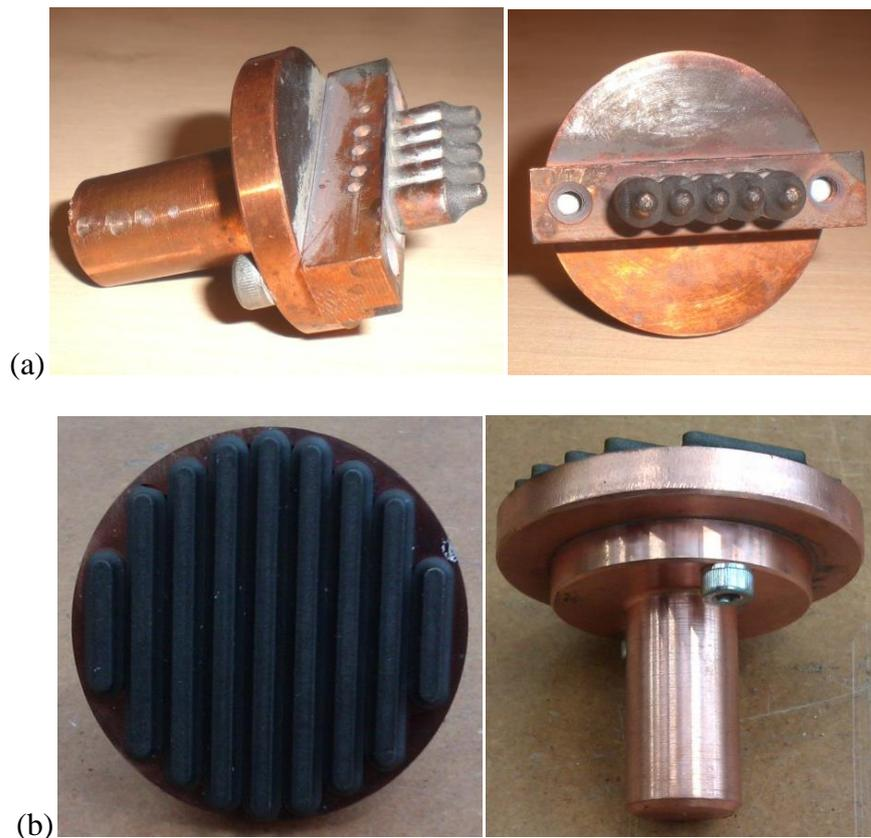
**Figure 3.13:** Different views of the fabricated tool for producing the T-HEX and the F-HEX edge shapes on the plate attachments.
