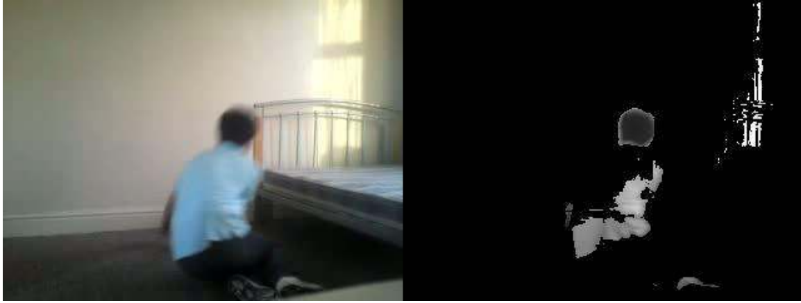
Figure 3.2 Background Subtracted Image using Approx. Median Filtering
